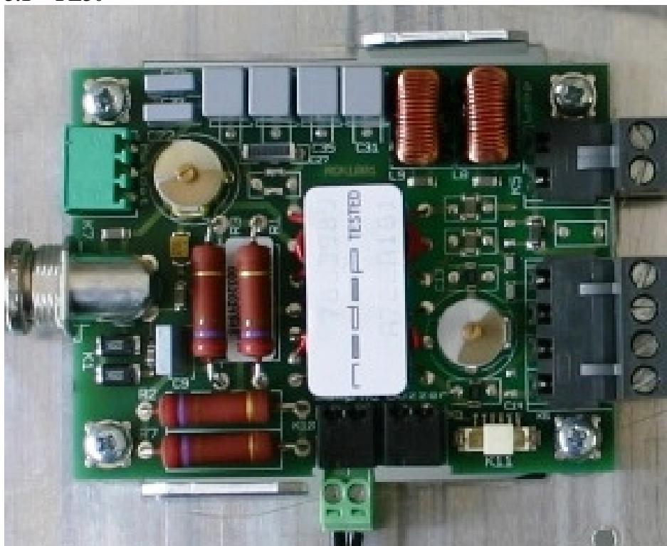
Description of EUT: Anti Pilferage System incl. Metal detection
