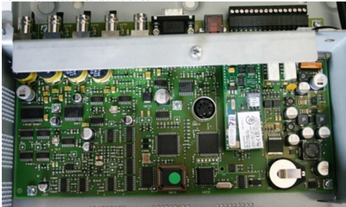
Description of EUT: Anti Pilferage System incl. Metal detection
