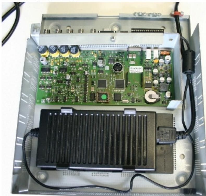
Description of EUT: Anti Pilferage System incl. Metal detection
