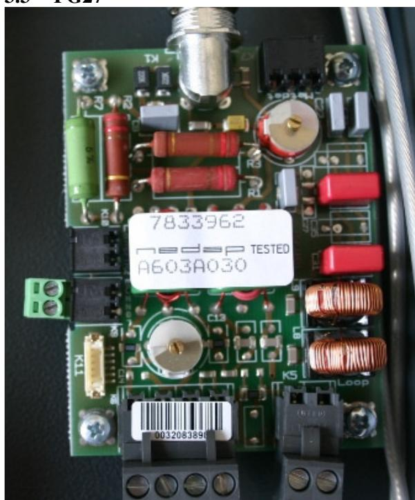
Description of EUT: Anti Pilferage System incl. Metal detection
