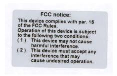
System unit NCC4 uses label below: The label size is 50mm (w) x 30 mm (h). The font size of the FCC ID is 8pt. The label is affixed on the side of the metal encasing. Page 2 of this document shows a drawing with the location indicated.
