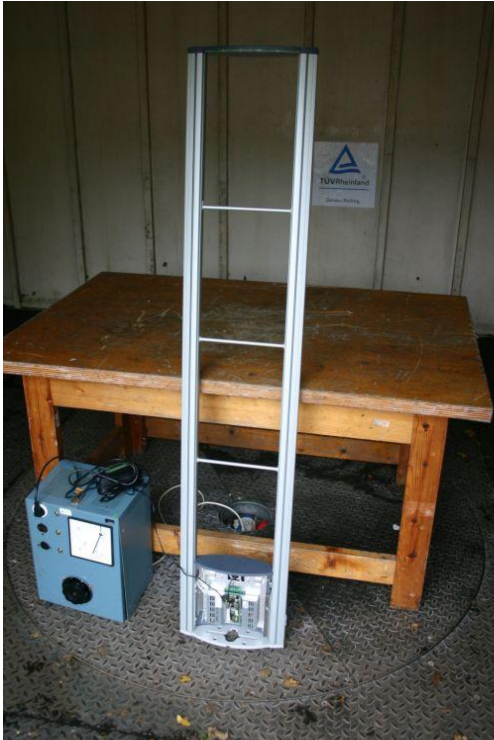
Photo showing setup EUT in typical installation (combination with ANT1 shown)
