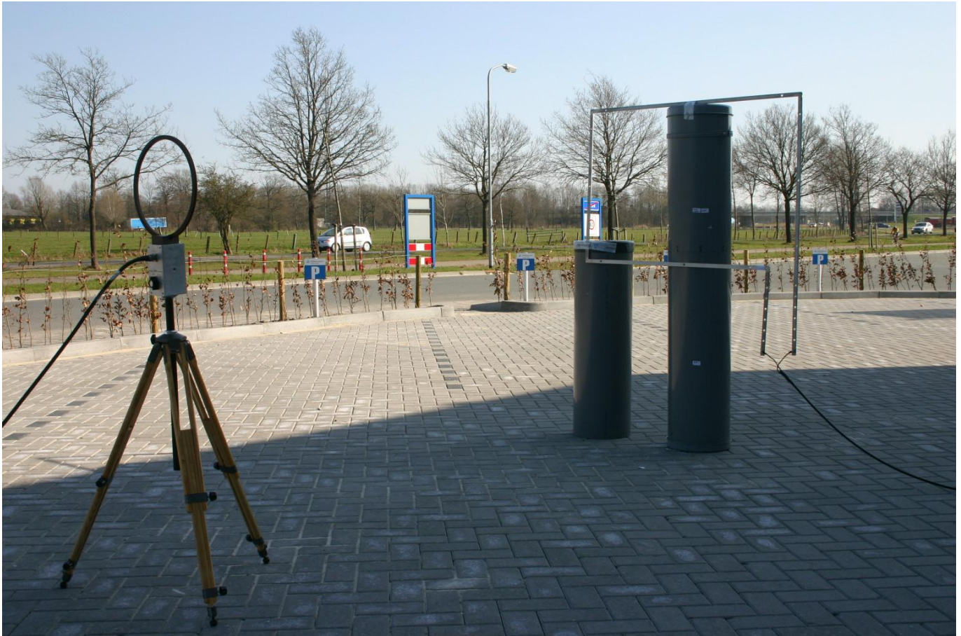
Measurement of magnetic field on the working frequency at 3 and 10 meters
