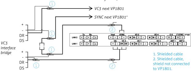
\*The SYNC connection is necessary for HDX ISO synchronization between other readers. For FDX a SYNC connection is possible, but not necessary if only one antenna is used. When two antennas are used the SYNC connection is always needed, even when FDX-only (no ISO) mode is enabled. The switching between the two antennas uses the ISO timing.
