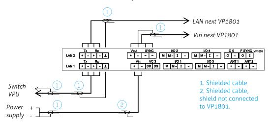
When connecting the Ethernet cable, the VP1801 automatically detects TX/RX, plus and minus connections, and switches to the correct connection.
