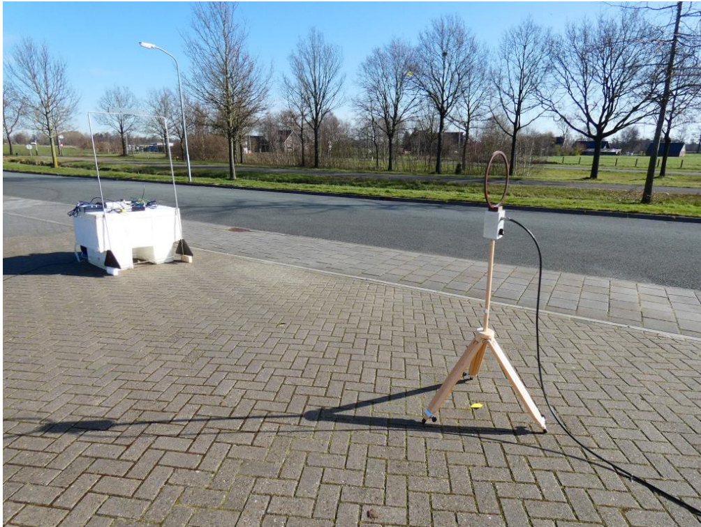
Setup EUT with Single Walk Through antenna, @5m
