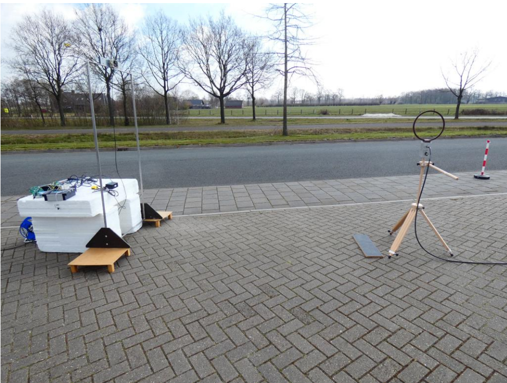
Setup EUT with Single Walk Through antenna, @3m (Y-orientation)
