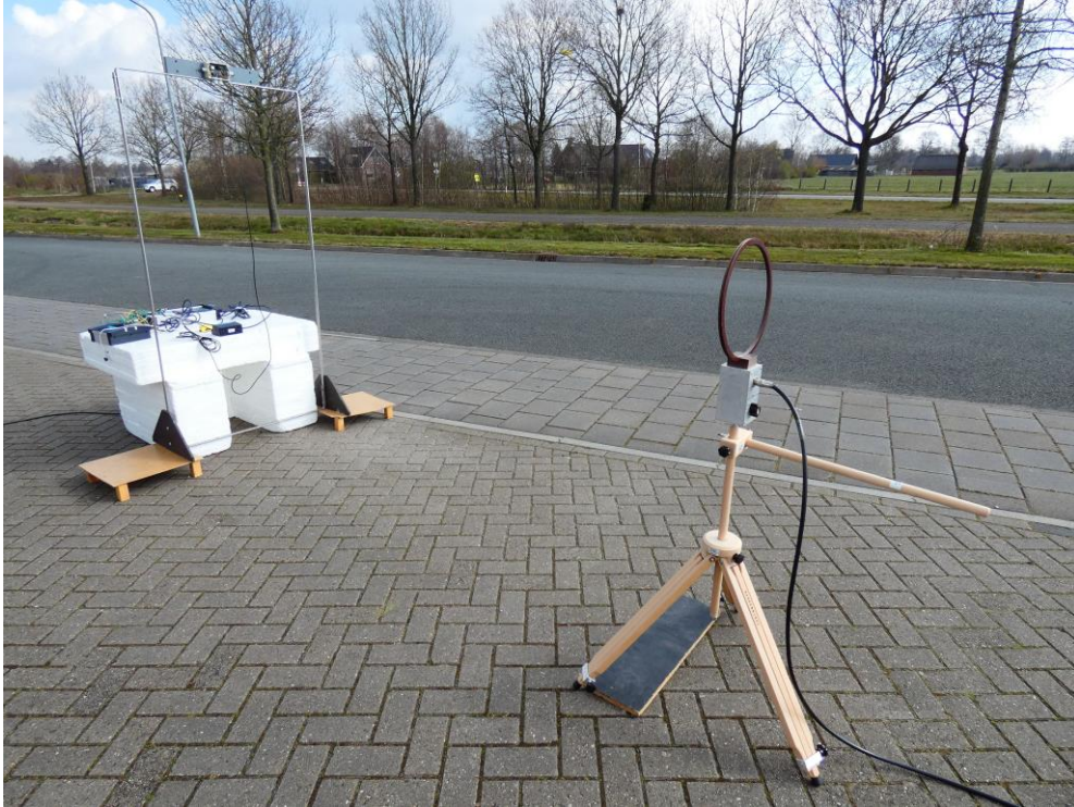
Setup EUT with Single Walk Through antenna, @3m (X-orientation)
