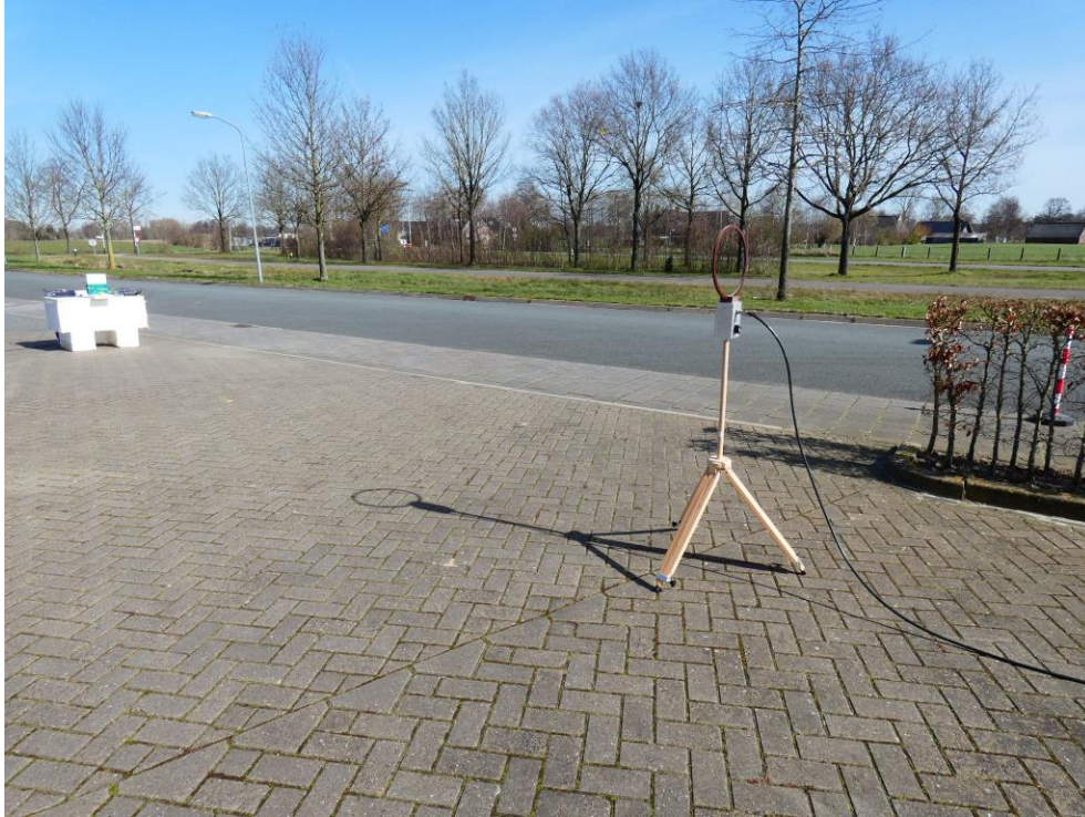
Setup EUT with VP6012 antenna @10m
