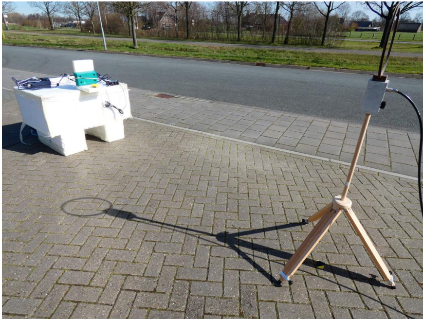
Setup EUT with VP6012 antenna @3m
