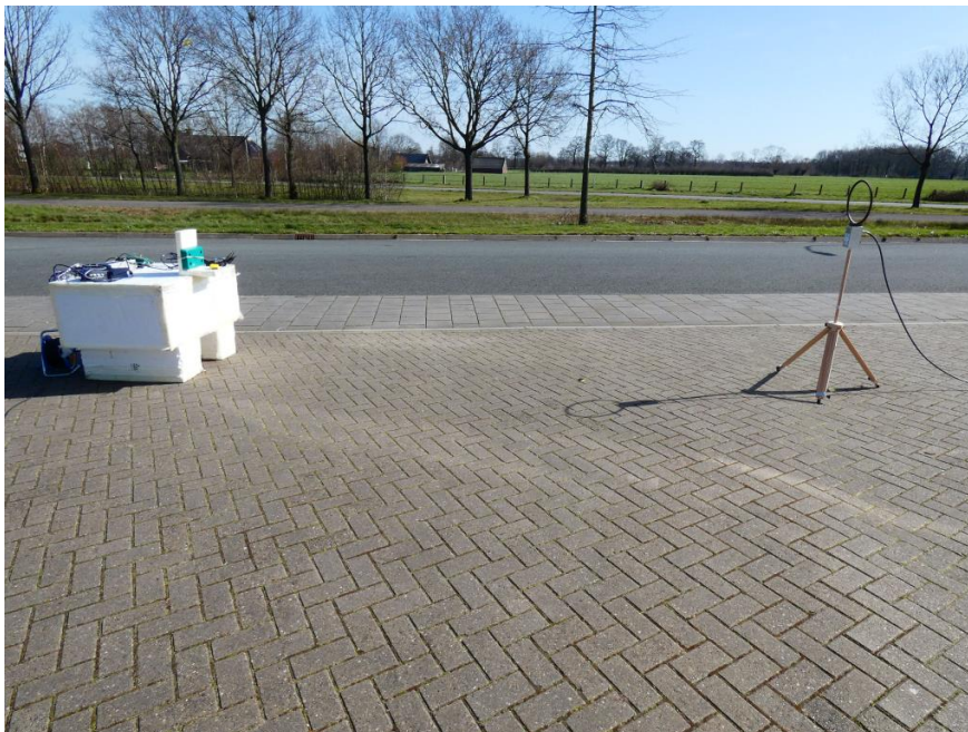
Setup EUT with VP6012 antenna @5m
