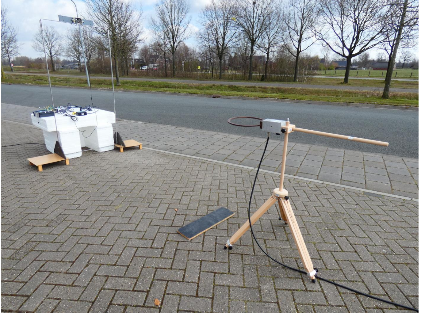
Setup EUT with Single Walk Through antenna, @3m (Z-orientation)
