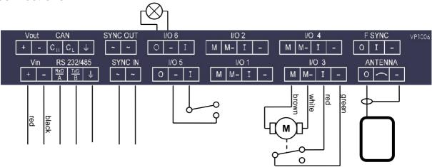
Figure above : motor, output and input is an example. Configuration is depending on the used behaviour components. Use display menu and push button to check and configure.
