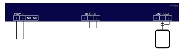
POWER + Input voltage from V-pack 24 VDC, +20% -20%
