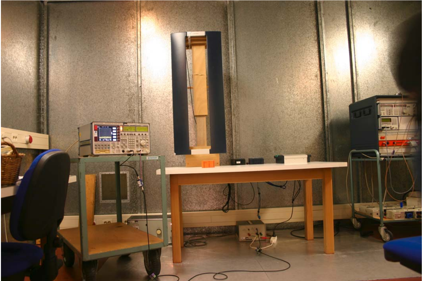
Photo 3: Conducted emission measurement set up; front side view.
