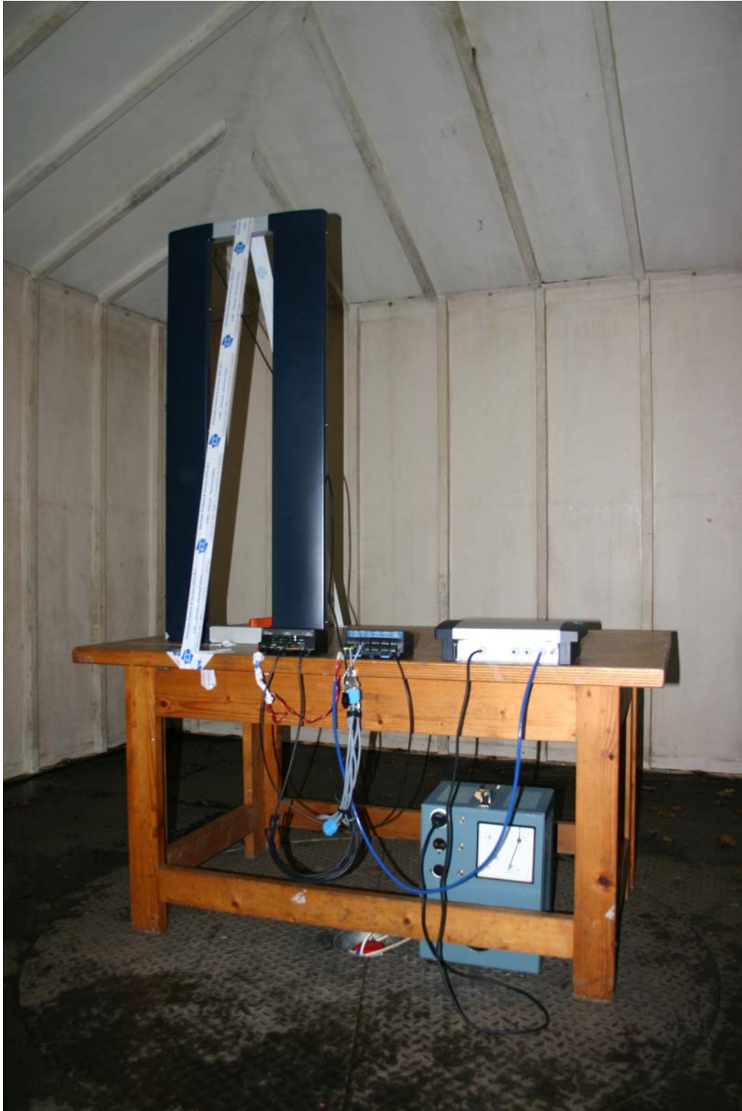
Photo 2: radiated emission measurement set up; back side view.
