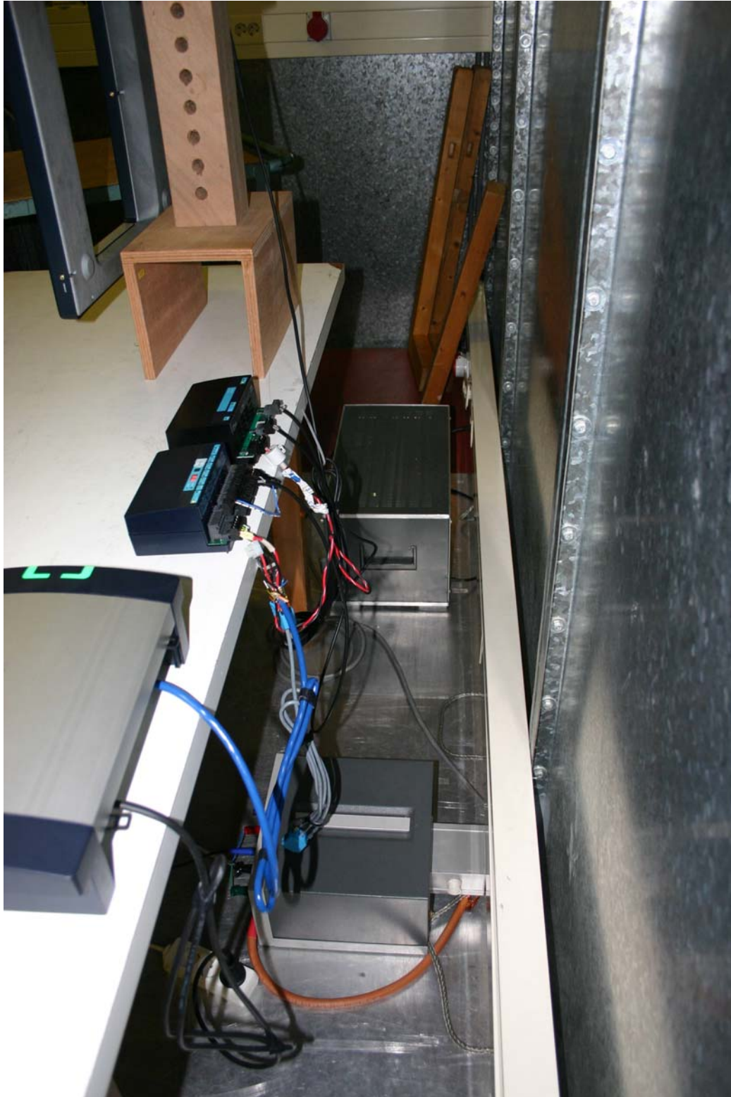
Photo 4: Conducted emission measurement set up; back side view.
