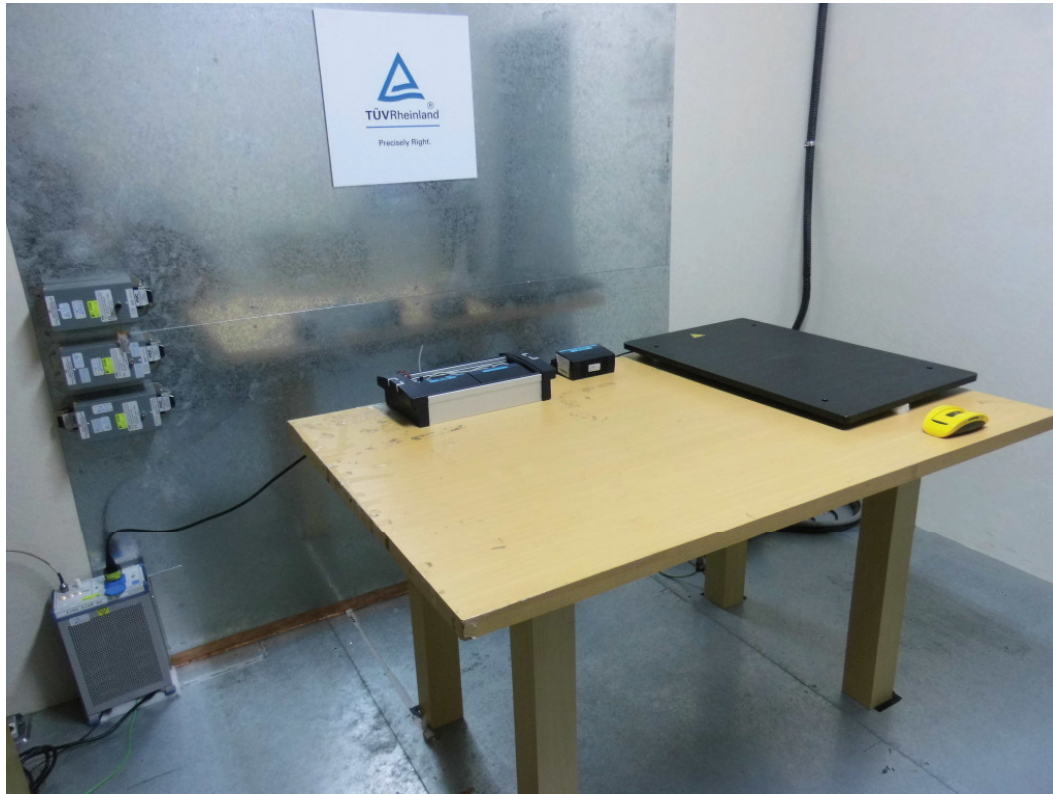
Photograph 9: Set-up for Mains Conducted testing Front_VP6042
