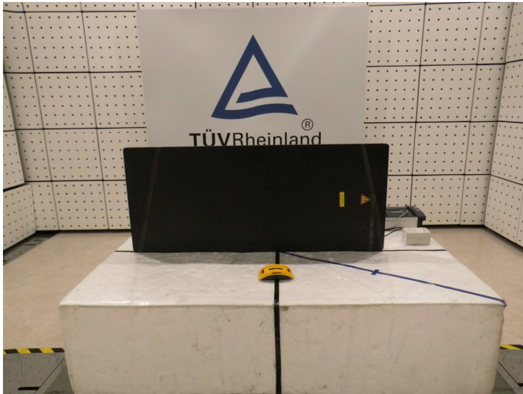
Photograph 11: Set-up for Spurious Emissions TX (Front View) Chamber_VP6050
