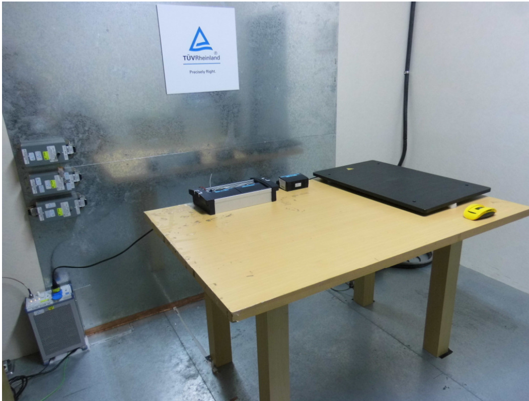
Photograph 9: Set-up for Mains Conducted testing Front_VP6042
