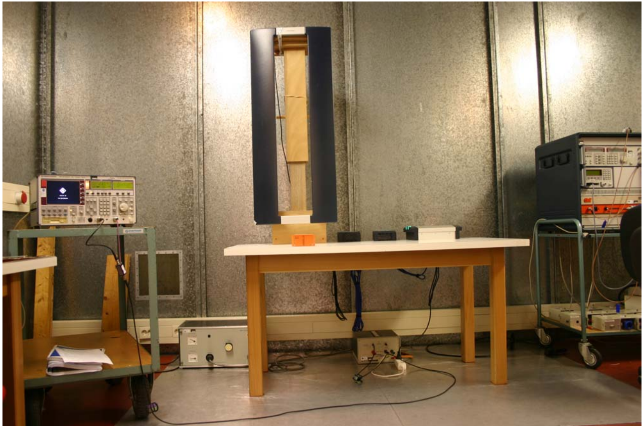
Photo 3: Conducted emission measurement set up VP1001, VP6001 front side view.
