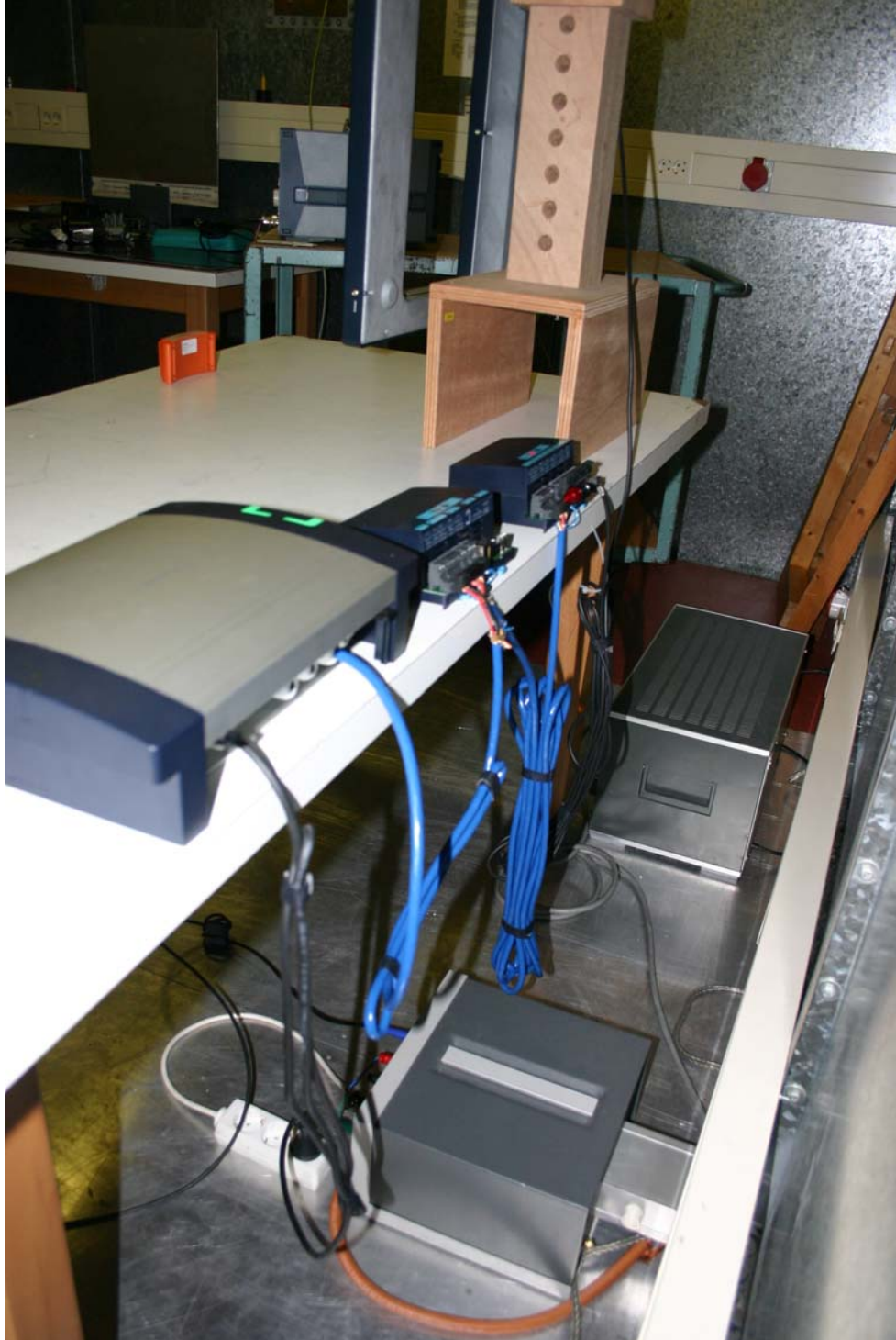
Photo 4: Conducted emission measurement set up VP1001, VP6001 back side view.
