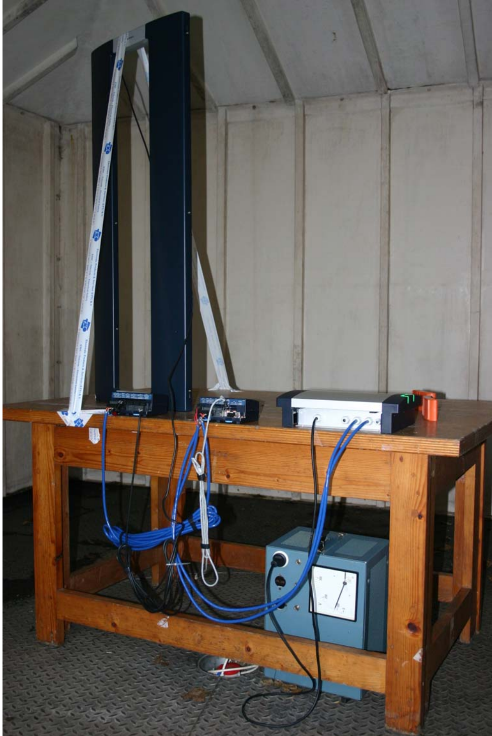
Photo 2: radiated emission measurement set up VP1001, VP6001 back side view.
