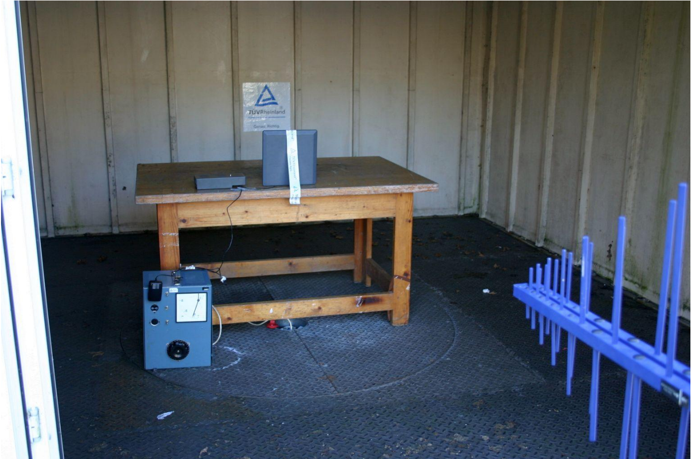
Radiated emission setup, Electric field
