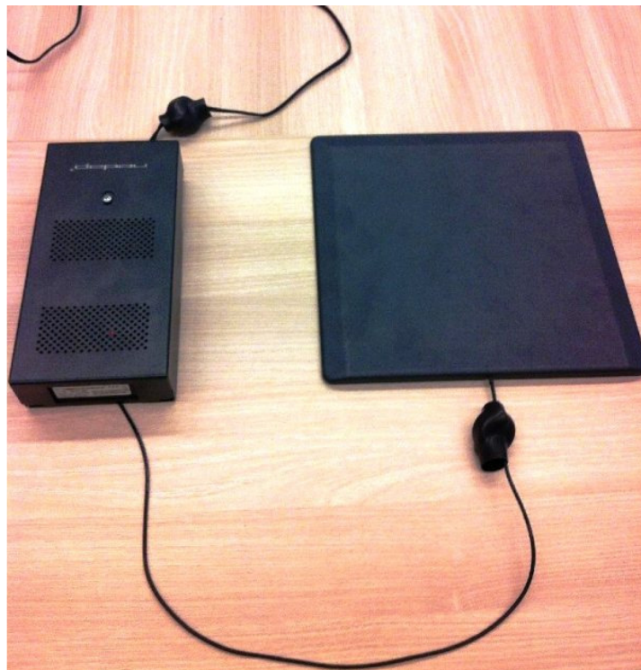
The finished solution with two ring cores provided in antenna – and power cable
