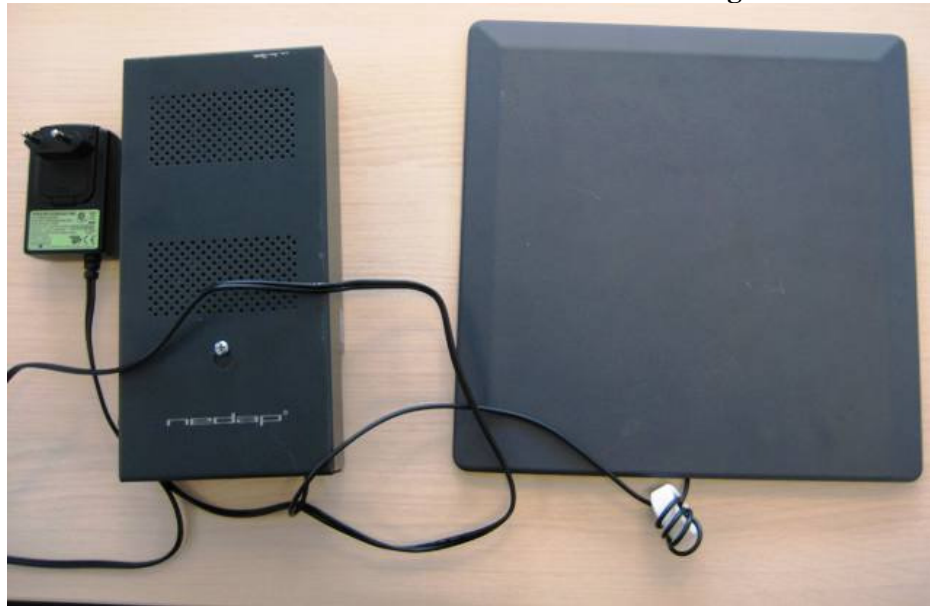
The finished solution with two ring cores provided in antenna – and power cable
