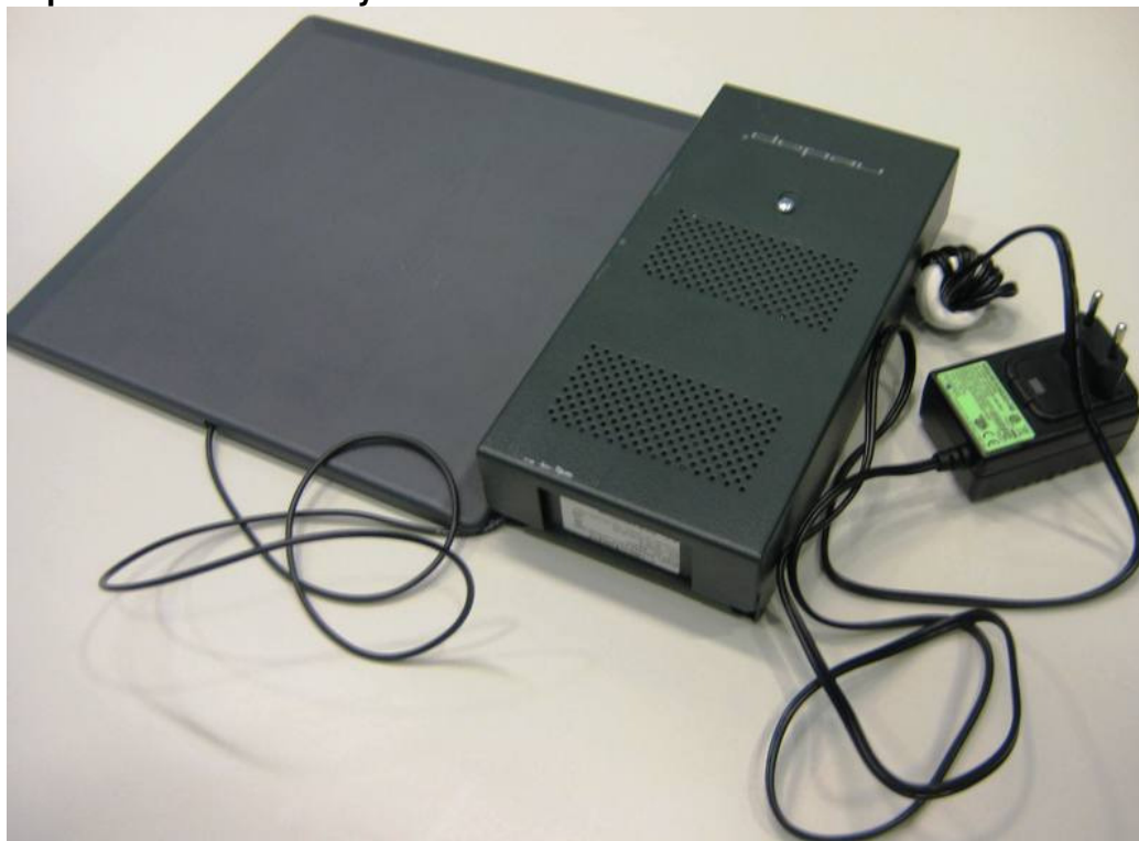
Ring core in power line only
