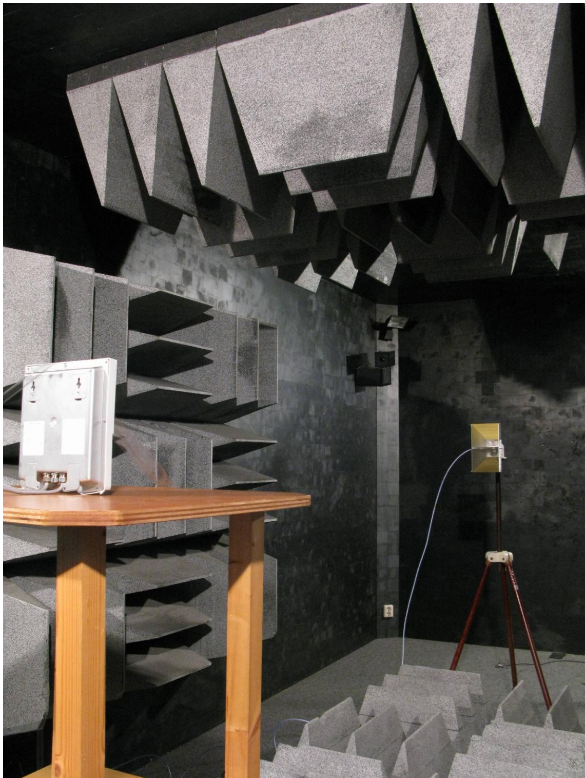
Photograph 2: Test setup radiated emissions (1 - 13 GHz)
