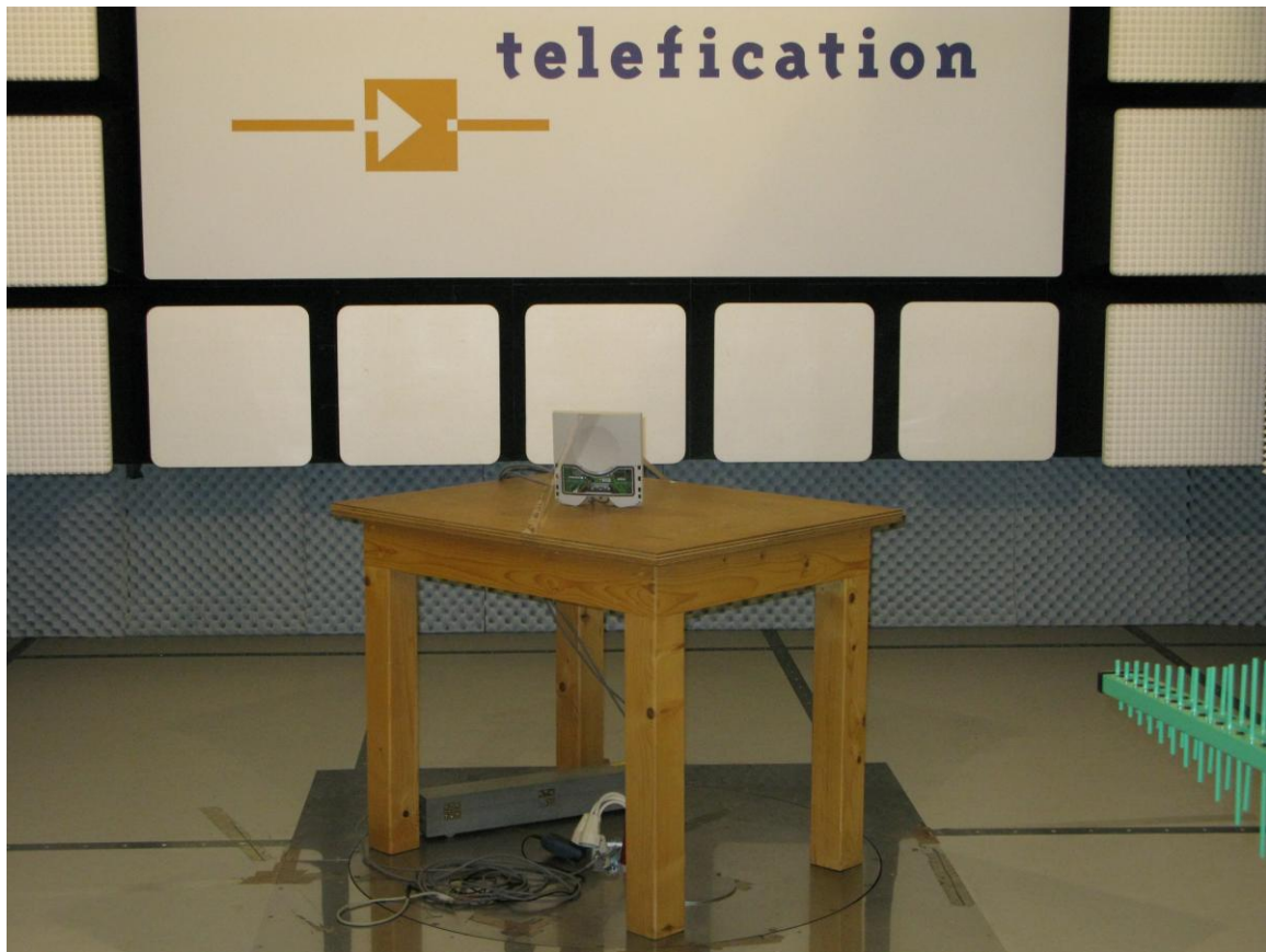
Photograph 1: Radiated emissions test setup (0.03 – 1 GHz)
