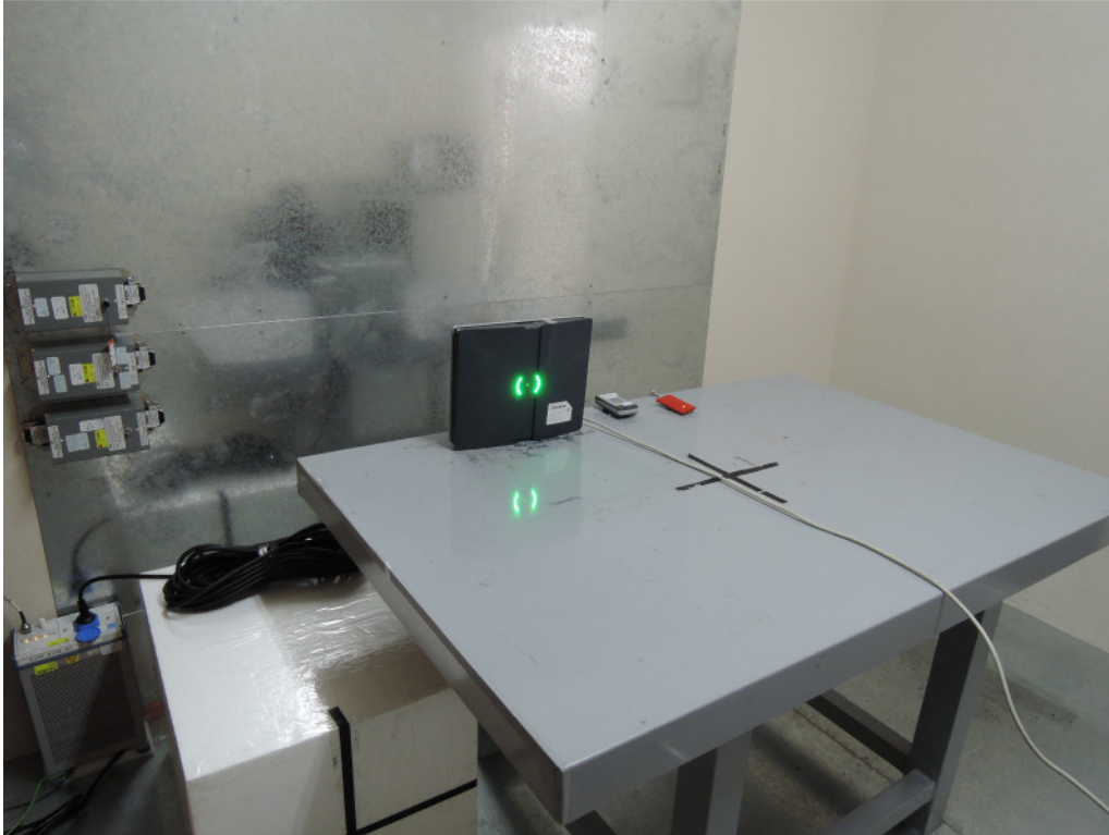
Photograph 4: Set-up for for Mains Conducted testing Back
