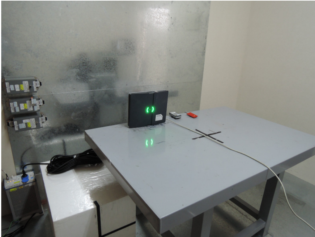
Photograph 4: Set-up for for Mains Conducted testing Back
