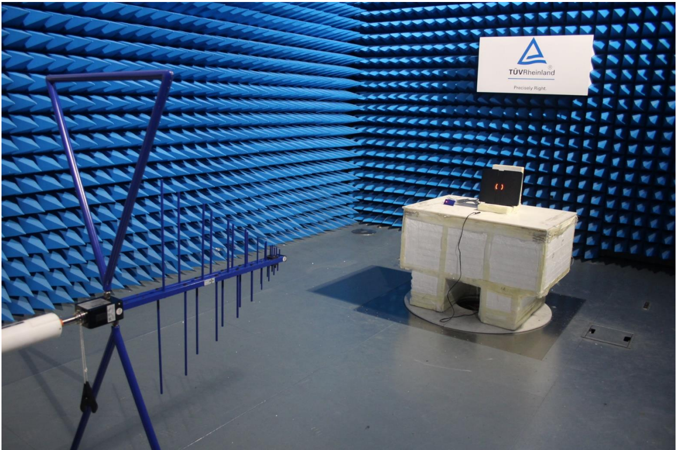
Setup EUT in Semi-AR, @3m
