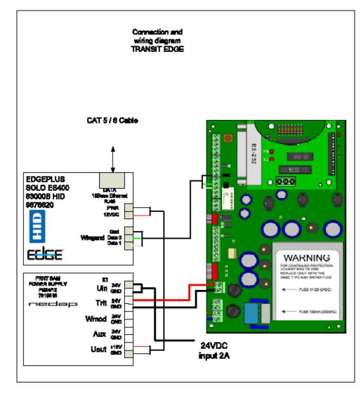
The diagram above shows schematically the internal connection between the used modules.
