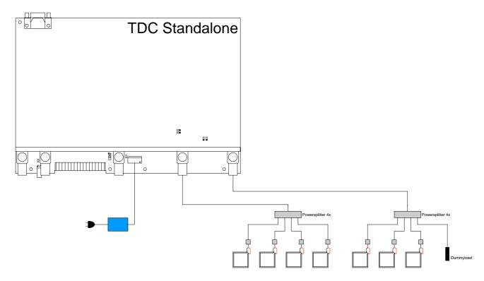
Example: TDC with 2 four way splitters, 7 add-on antenna's and 7 TDC Ducs or 7 TDC Buzducs and a dummyload for the last channel
