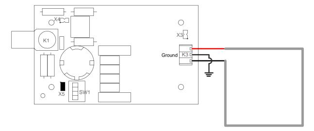
The DUC is used to connect an O-shape antenna to a deactivator.
