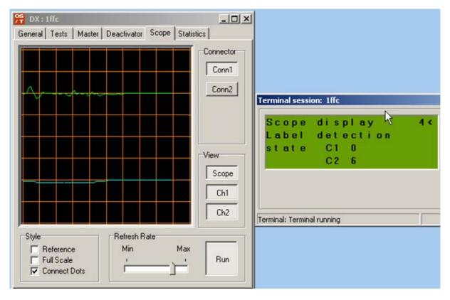
At the terminal screen (7-7-2) use the options 3 or 4 to view the directional coupler signal.
