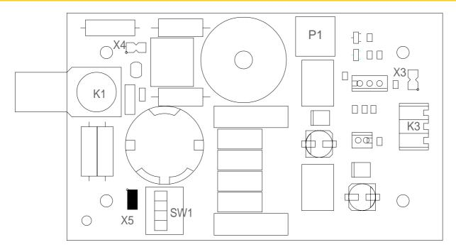
The TDC Buzduc is a combination of the TDC Duc and TDC Buzzer. With the TDC Buzduc a hand- or flatbed scanner antenna with a local buzzer can be realized. The DUC is meant to connect an O-shape antenna to a deactivator.
