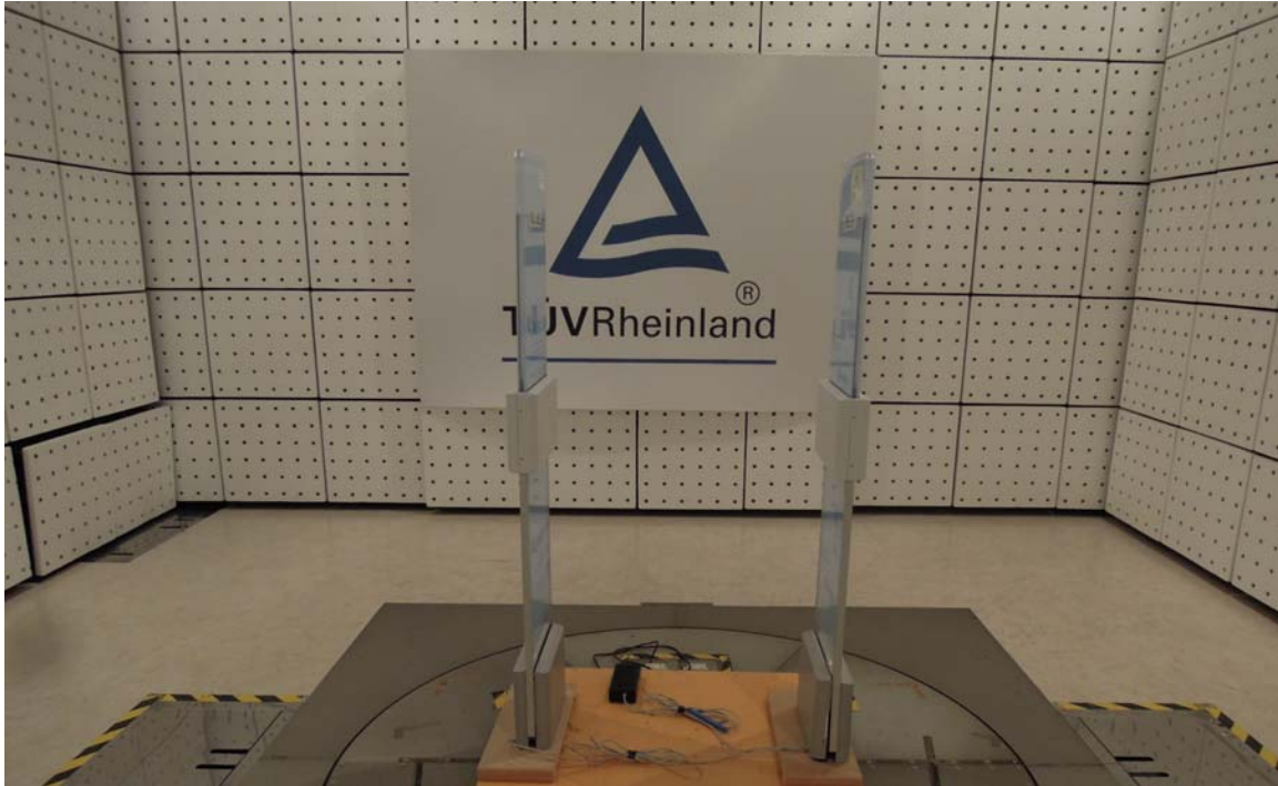
Photograph 1: Set-up for Radiated Emissions TX (Front View)
