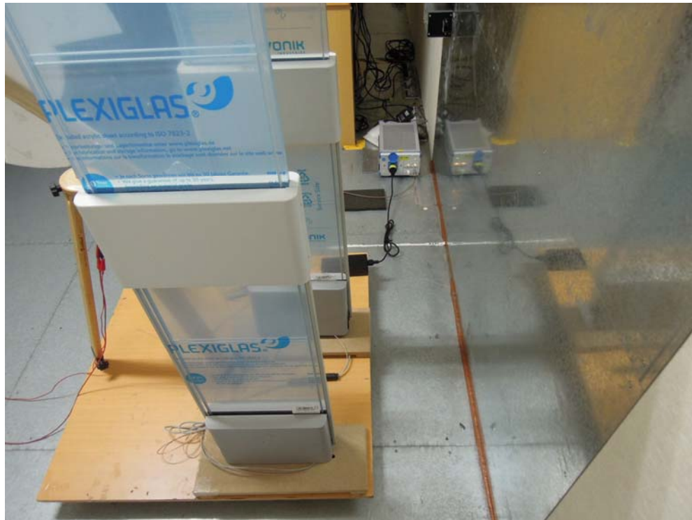
Photograph 4: Set-up for Mains Conducted testing Back
