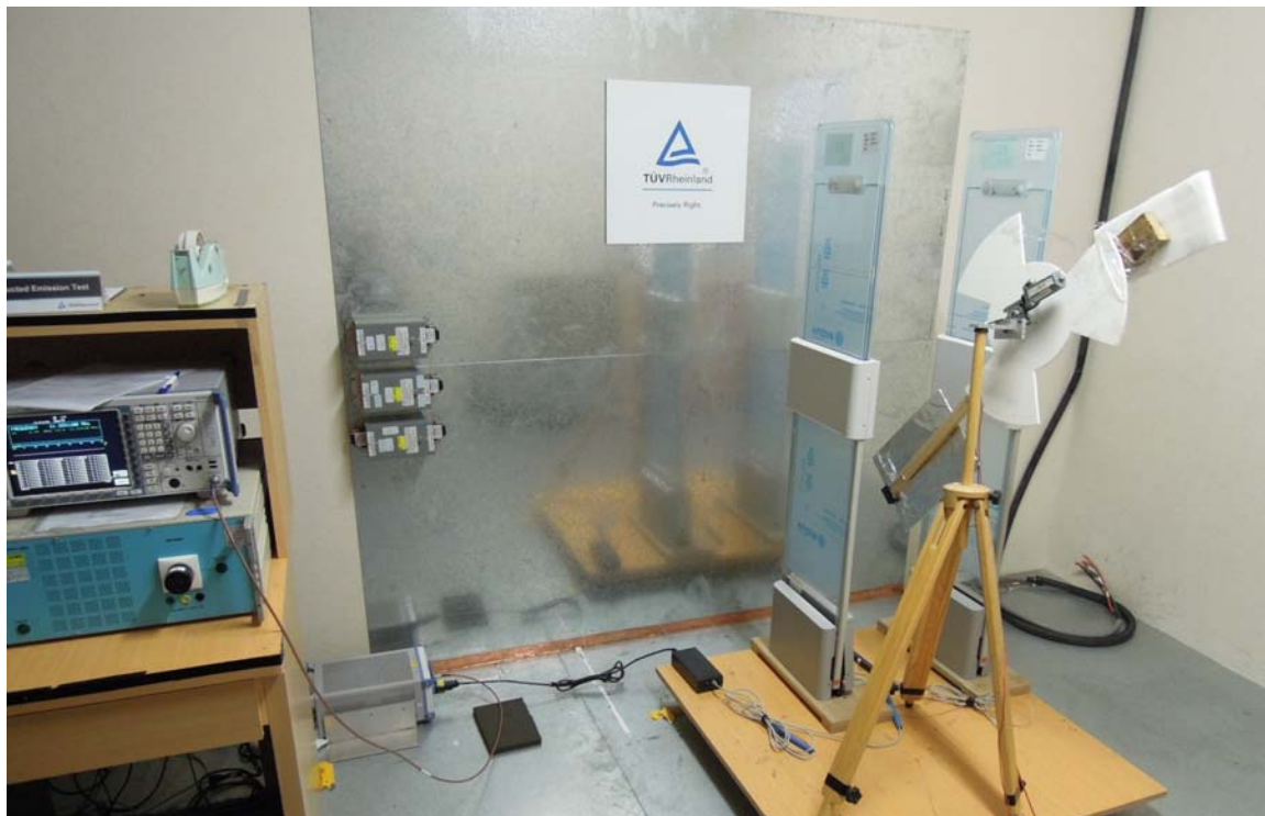
Photograph 5: Set-up for Mains Conducted testing Front
