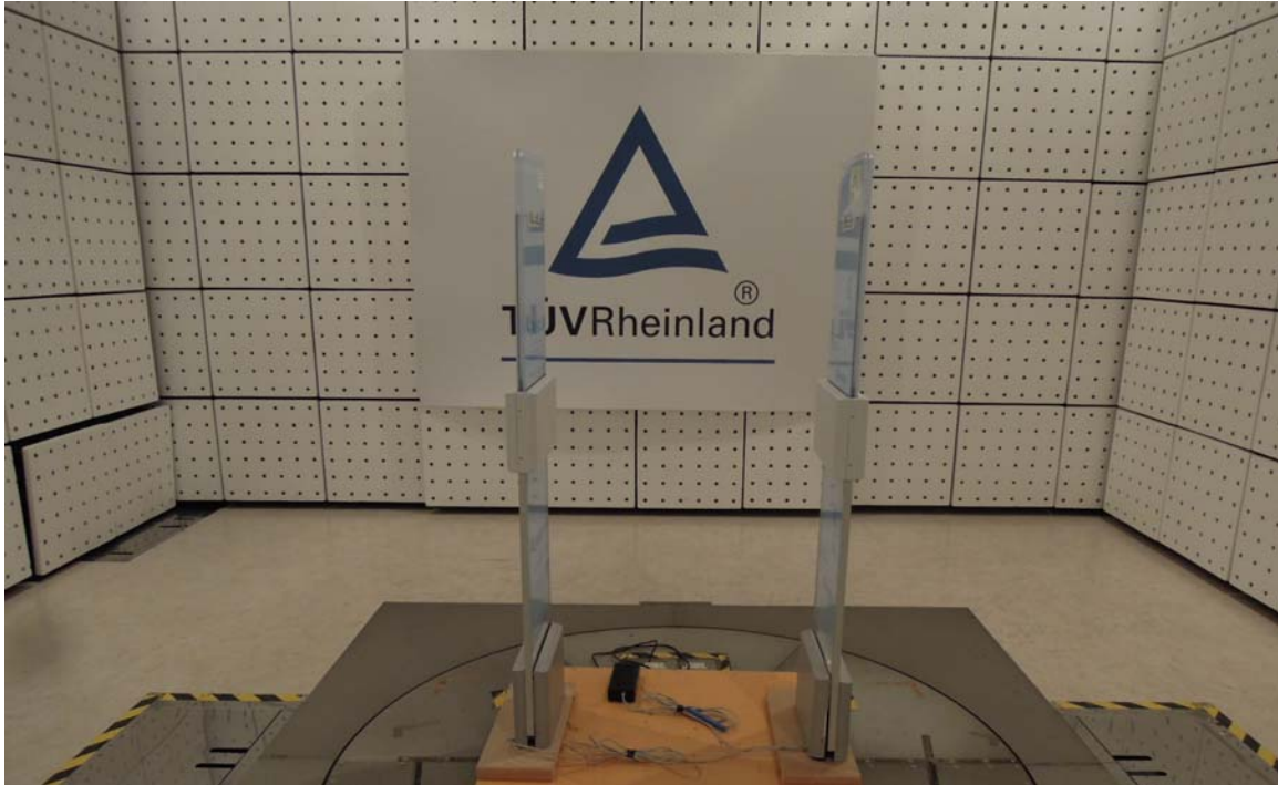
Photograph 1: Set-up for Radiated Emissions TX (Front View)
