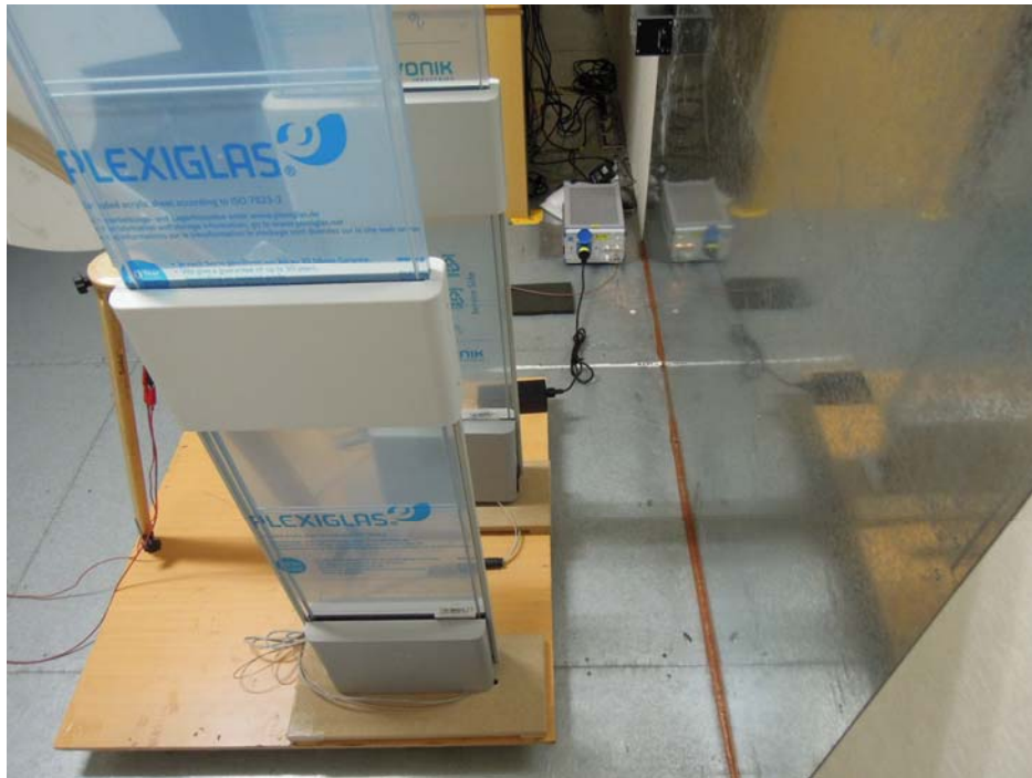
Photograph 4: Set-up for for Mains Conducted testing Back
