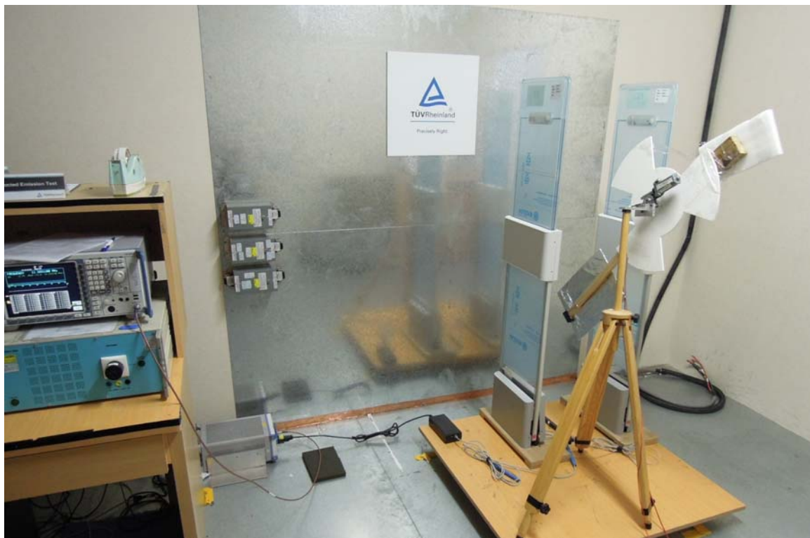
Photograph 5: Set-up for for Mains Conducted testing Front
