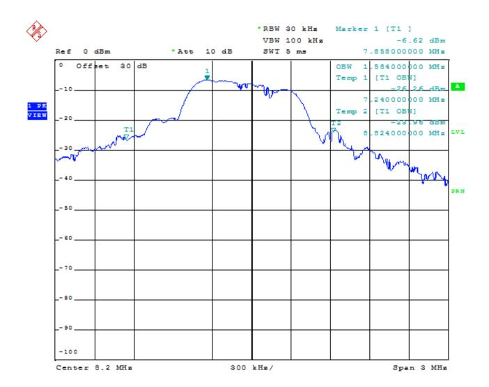
Plot1b: plot of the 99% emission bandwidth. Measured value is 1584 kHz as measured on a spectrum analyzer.
