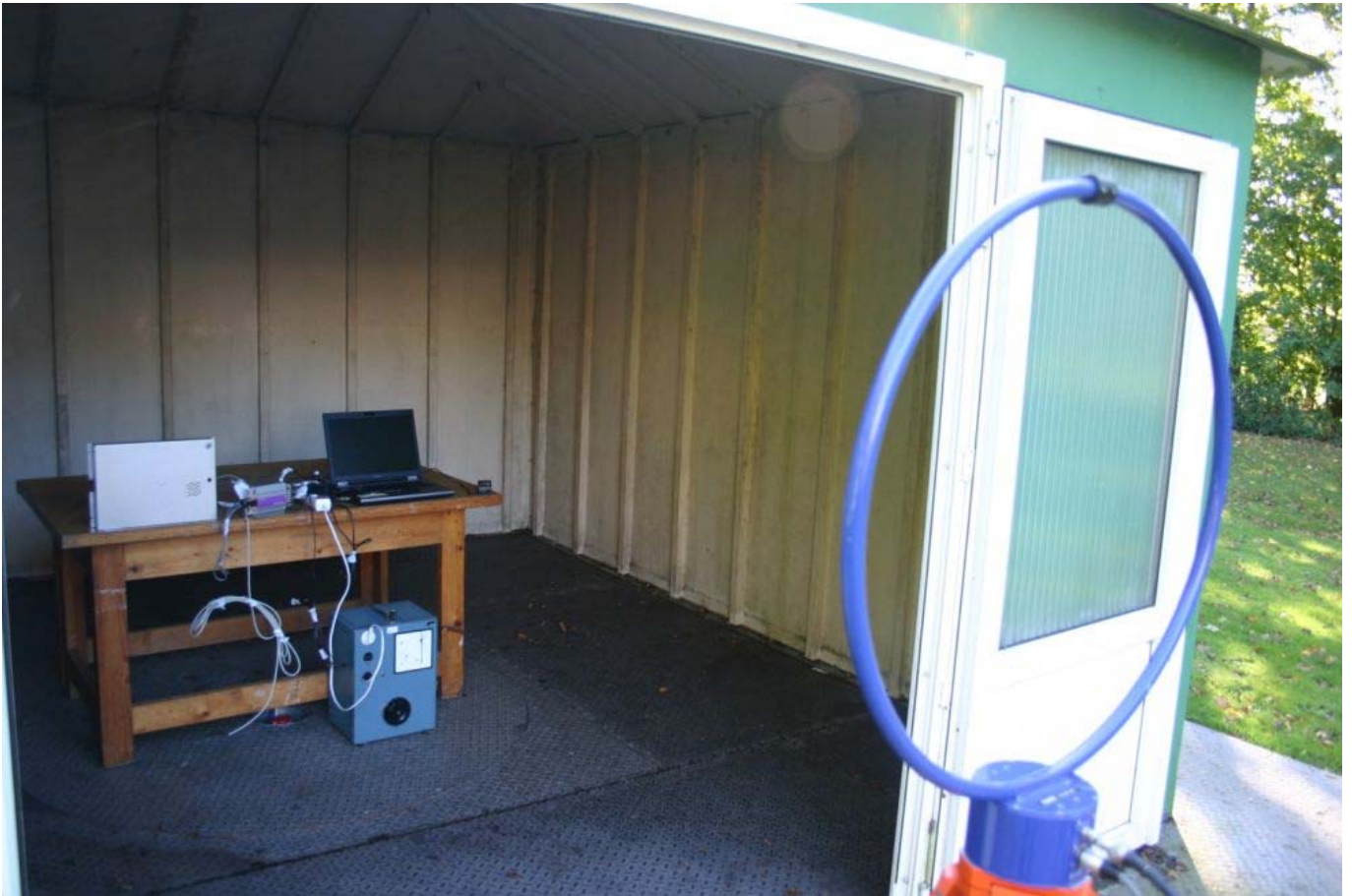
Typical setup for all combinations of EUT and Auxiliary equipment (EUT Vertical and Aux2 vertical, shown as example)
