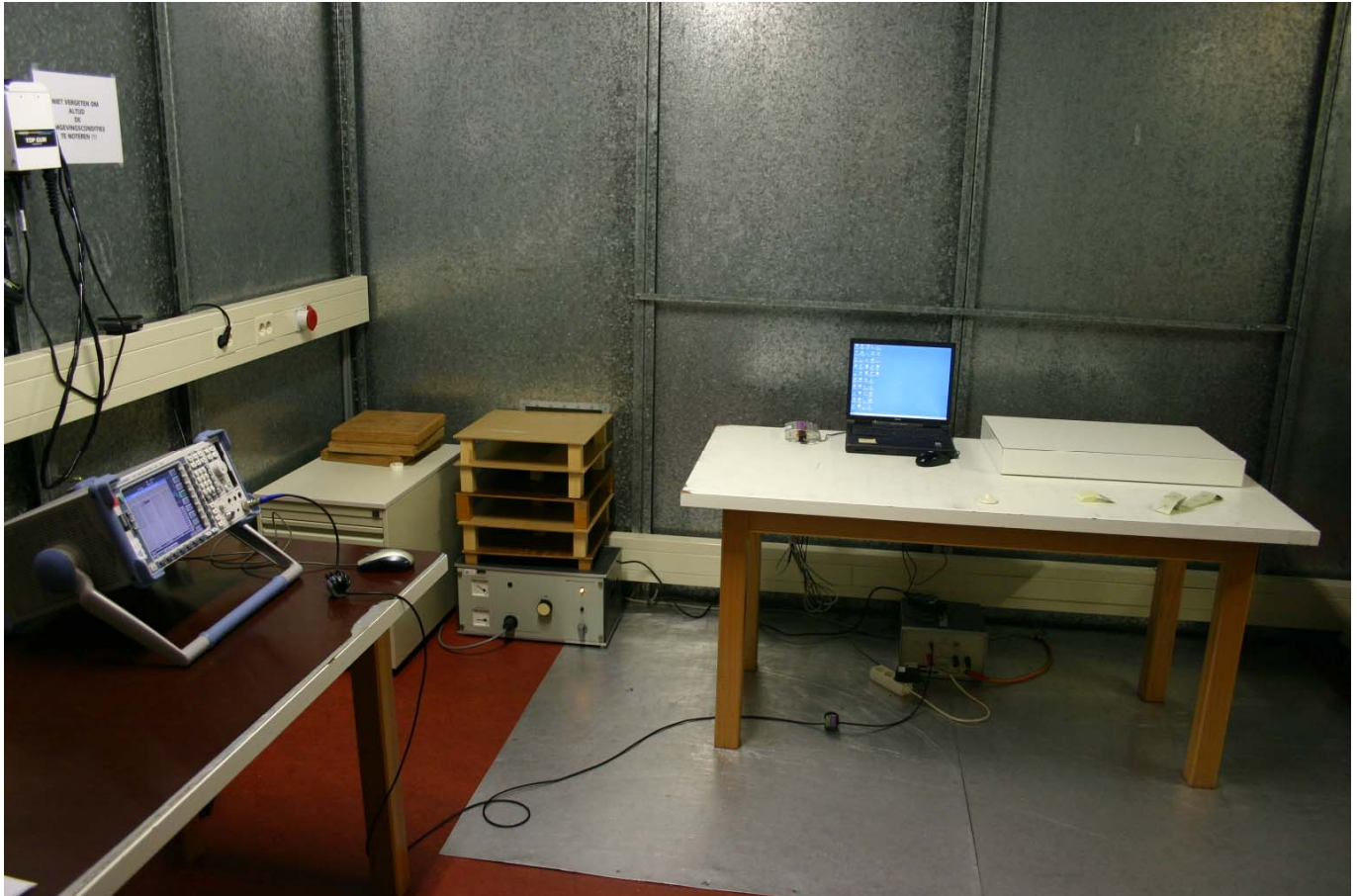
Typical setup for all combinations of EUT and Auxiliary equipment (EUT and Aux1, shown as example)
