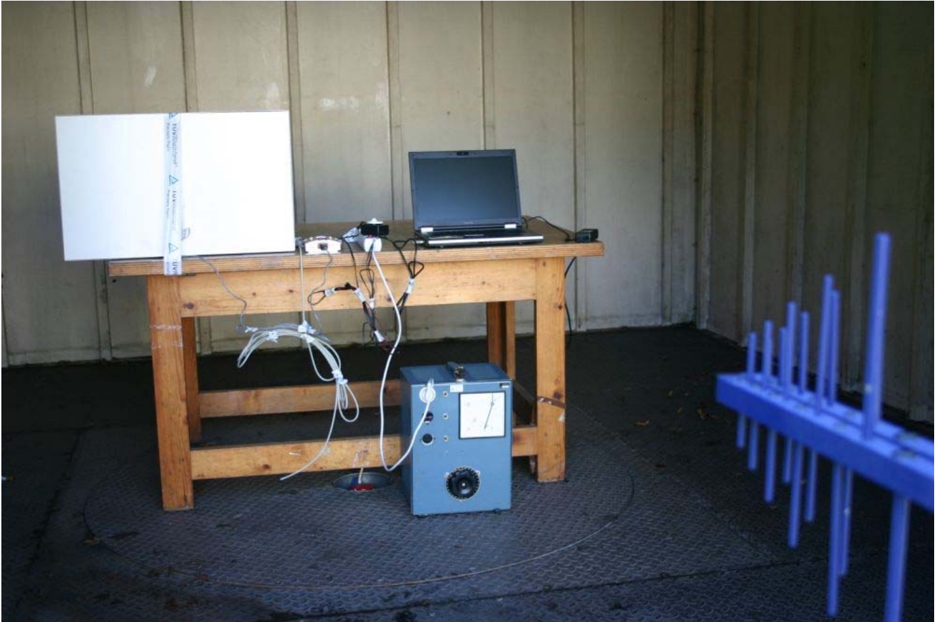
Typical setup for all combinations of EUT and Auxiliary equipment (EUT Horizontal and Aux1 vertical, shown as example)
