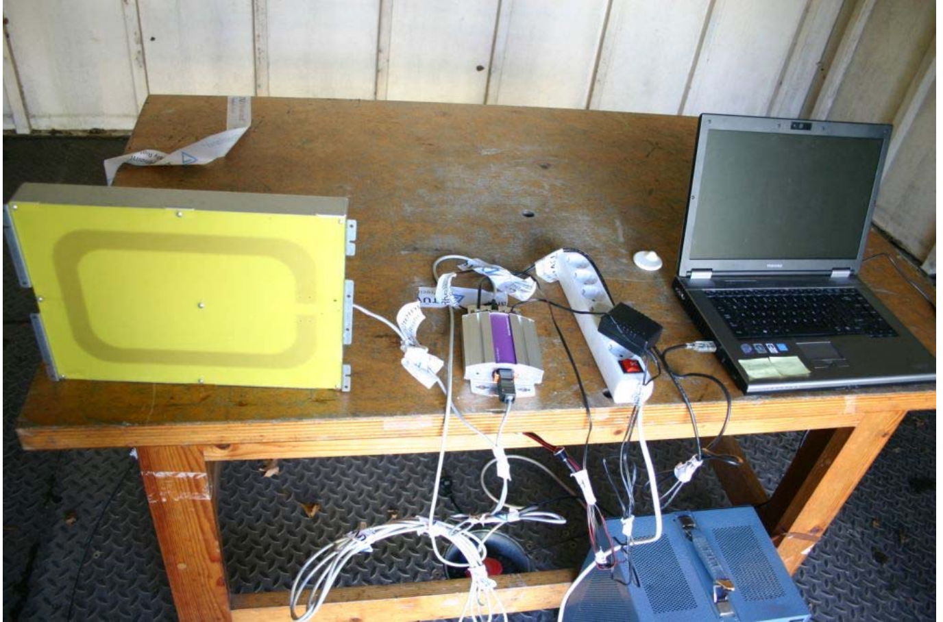
Typical setup for all combinations of EUT and Auxiliary equipment (EUT Horizontal and Aux2 Vertical, shown as example)
