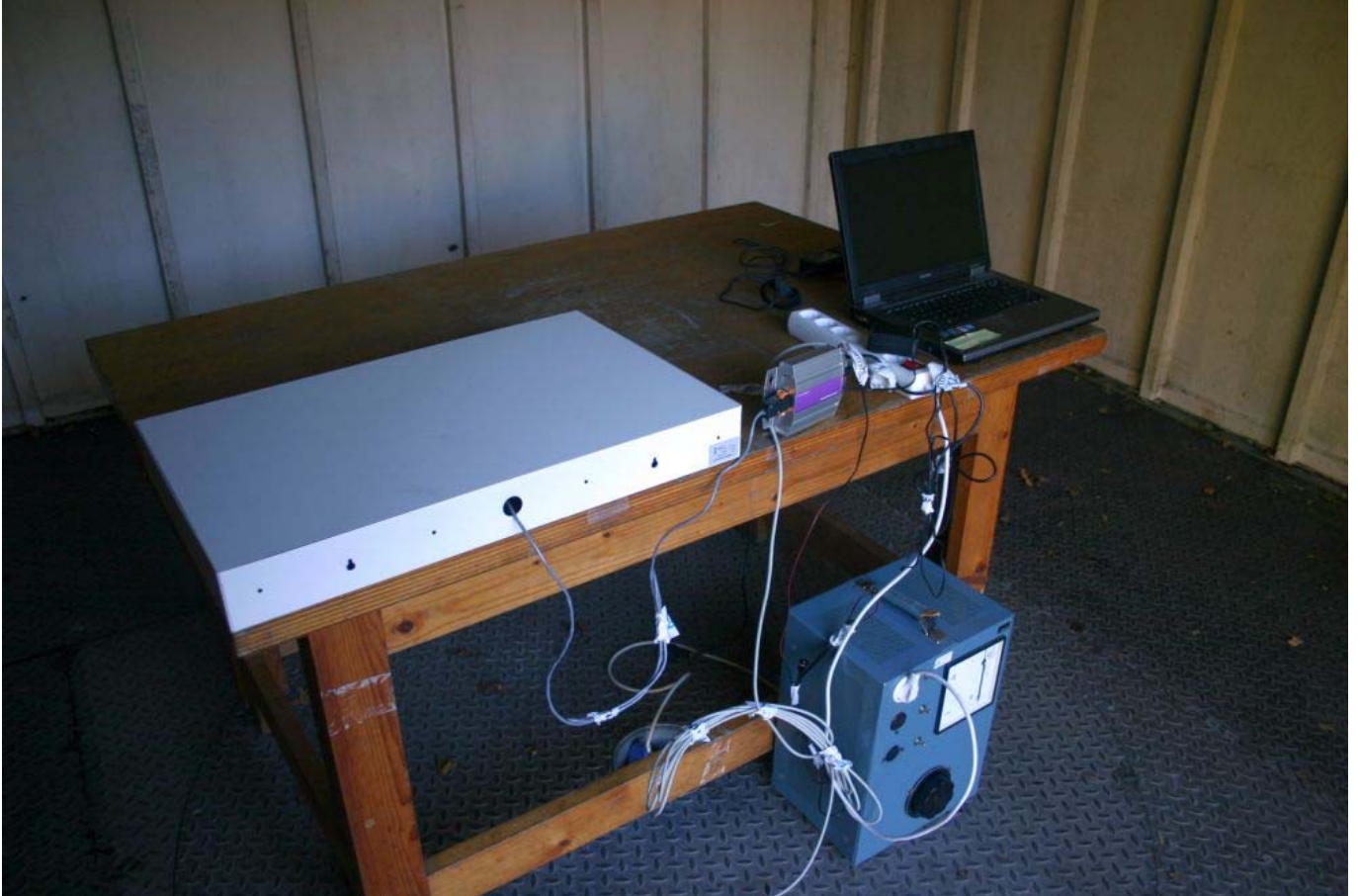
Typical setup for all combinations of EUT and Auxiliary equipment (EUT Vertical and Aux1 Horizontal, shown as example)
