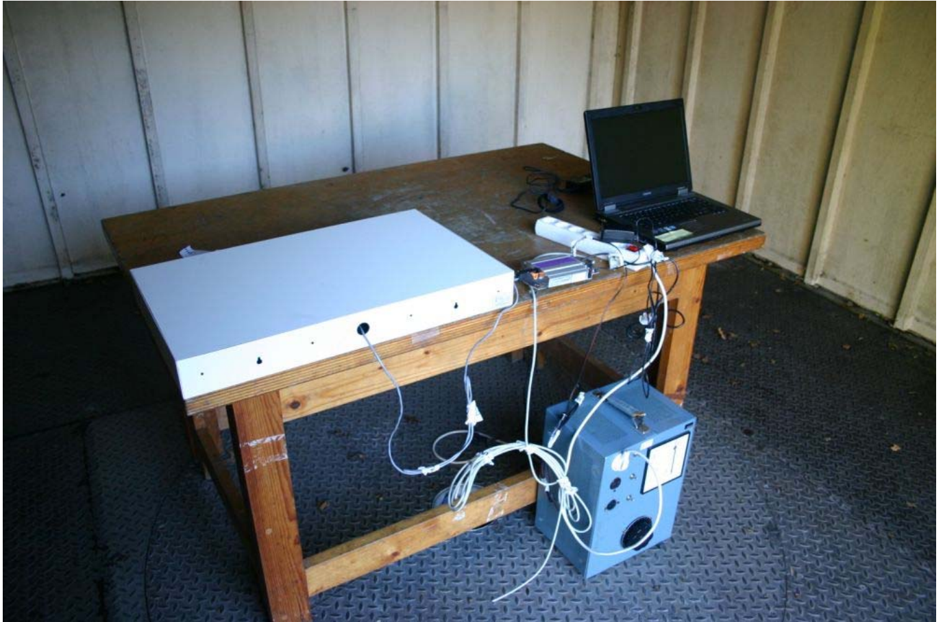
Typical setup for all combinations of EUT and Auxiliary equipment (EUT Horizontal and Aux1 Horizontal, shown as example)
