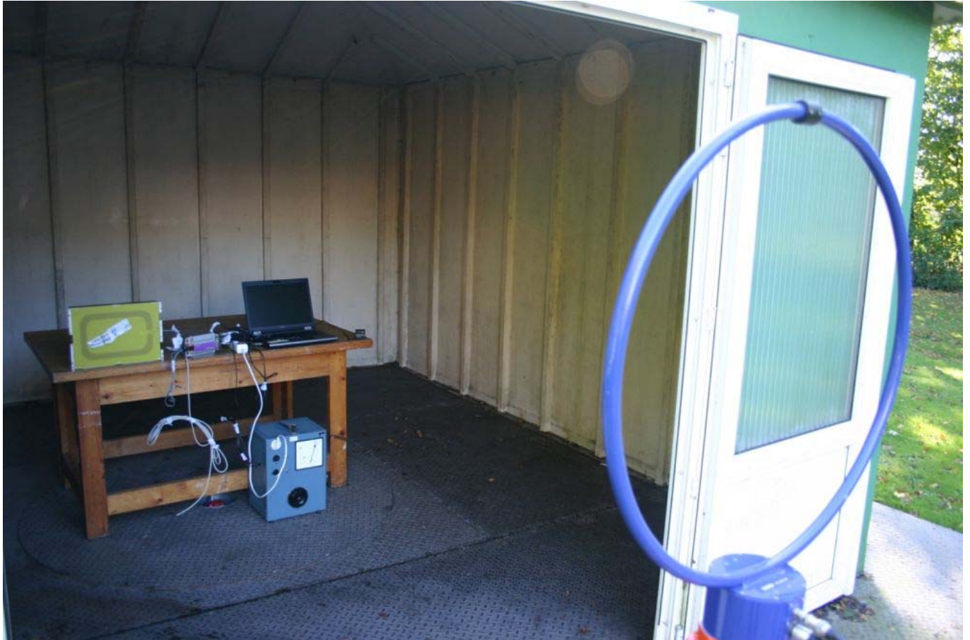
Typical setup for all combinations of EUT and Auxiliary equipment (EUT Vertical and Aux2 vertical-rotated, shown as example)
