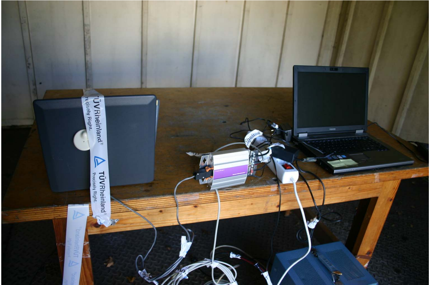
Typical setup for all combinations of EUT and Auxiliary equipment (EUT Vertical and Aux3 Vertical, shown as example)
