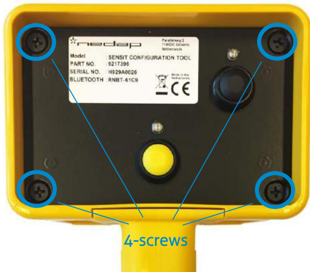
Figure 18: Configuration tool remove screws to open housing
