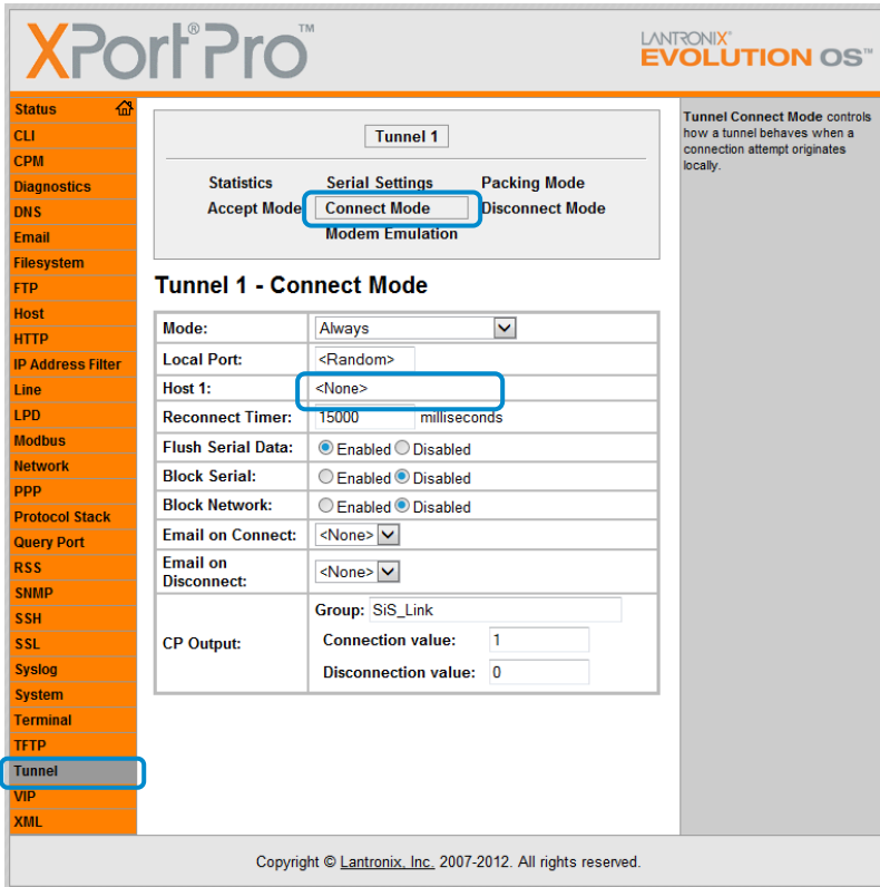
Figure 25: SENSIT Gateway TCP/IP Tunnel configuration
