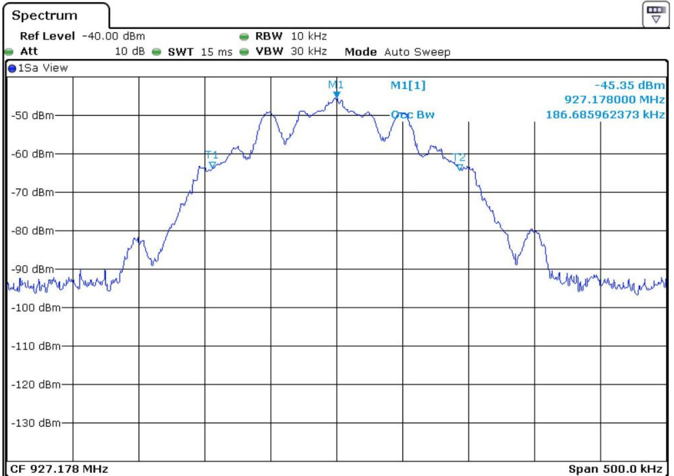
Plot 3: Occupied 20dB Bandwidth (= 186.7 kHz) of the EUT transmitting at 927.2 MHz
