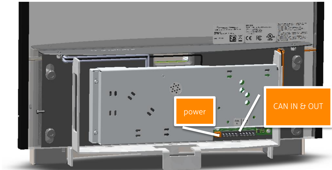
Figure 19 - PG45i match PCB location
