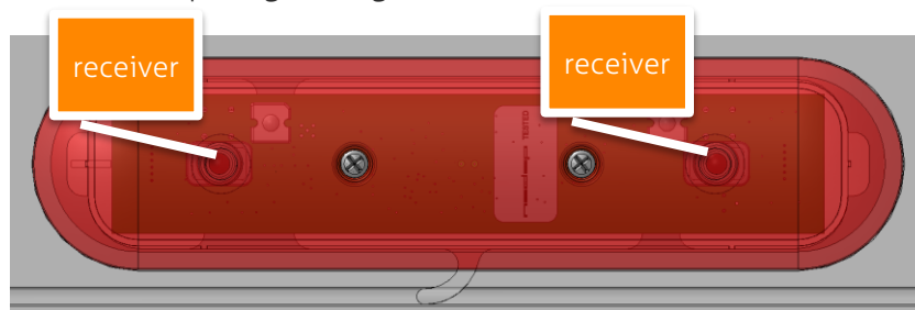
Figure 7 - receiver side of customer counting module
