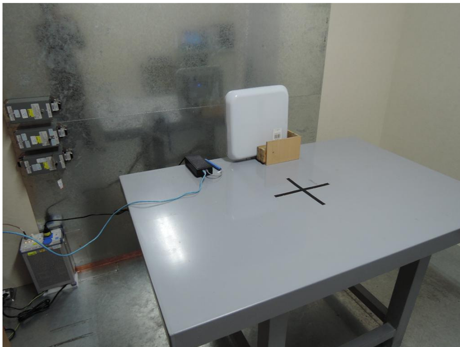
Photograph 5: Set-up for for Mains Conducted testing Front
