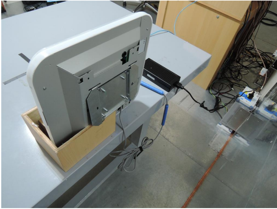
Photograph 4: Set-up for for Mains Conducted testing Back
