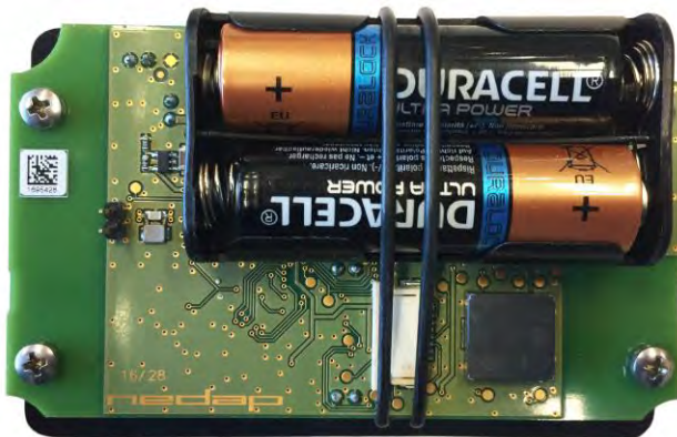
Figure 19: Configuration tool: Battery replacement
