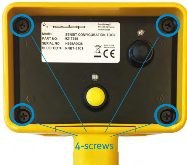
Figure 18: Configuration tool remove screws to open housing
