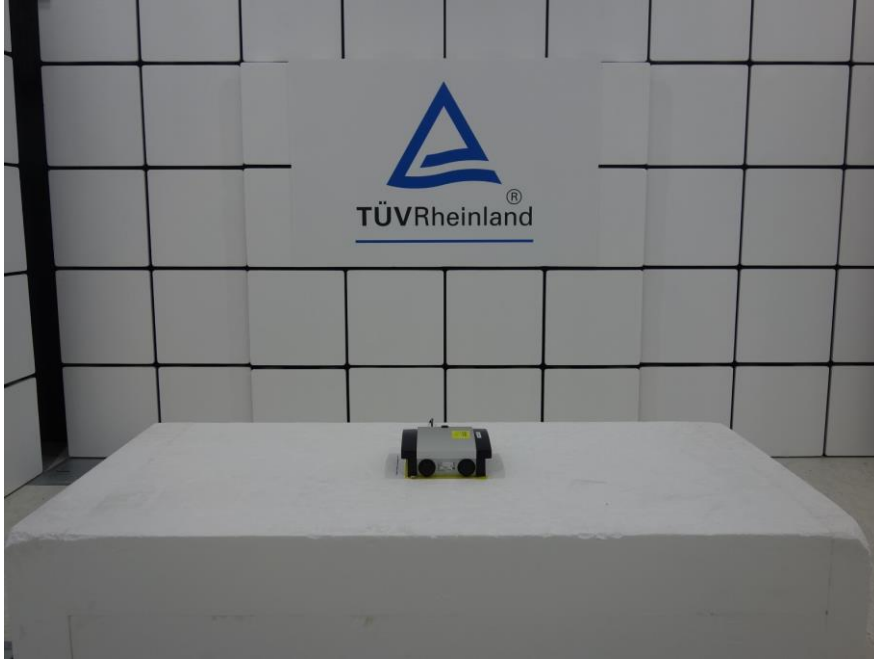
Photograph 2: Test Setup for Spurious Emissions (Front View 2)
