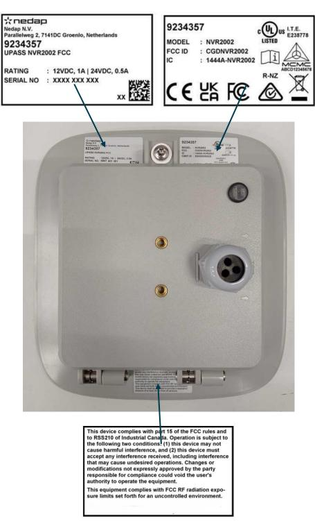
Fig.7 – Rear view of NVR2002, including location of labels
