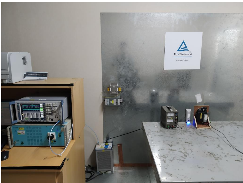
Photograph 6: Set-up for AC mains (Front View)
