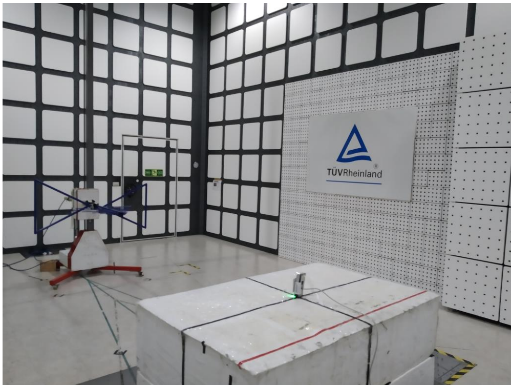
Photograph 2: Set-up for Spurious Emissions (Back View 1)
