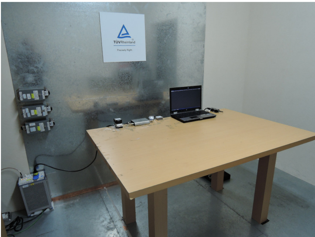
Photograph 5: Set-up for Mains Conducted testing Front
