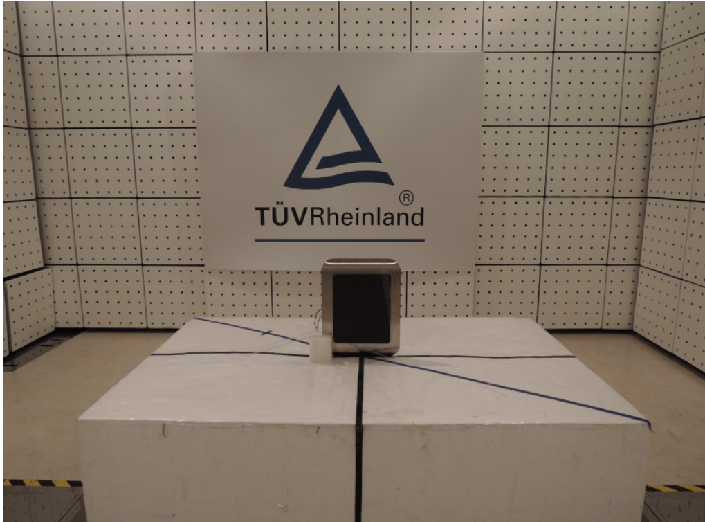
Photograph 1: Set-up for Spurious Emissions TX (Front View)
