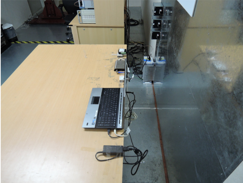
Photograph 4: Set-up for for Mains Conducted testing Back
