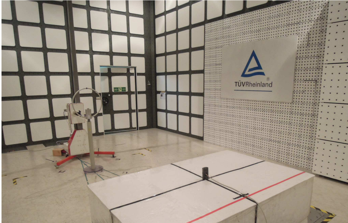
Photograph 3: Set-up for Spurious Emissions (Back View 2)
