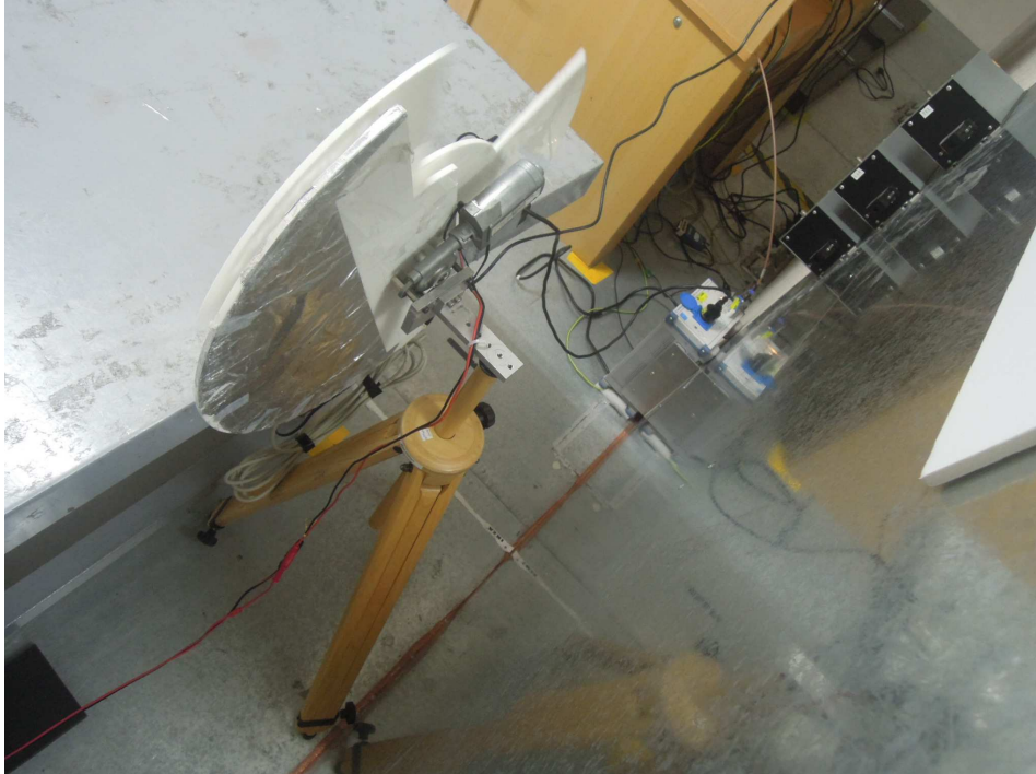
Photograph 4: Set-up for for Mains Conducted testing Back
