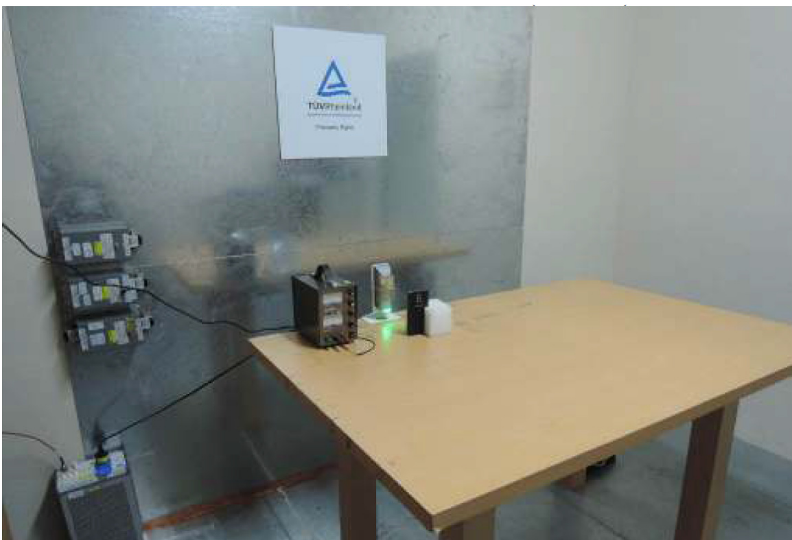
Photograph 5: Set-up for for Mains Conducted testing Front
