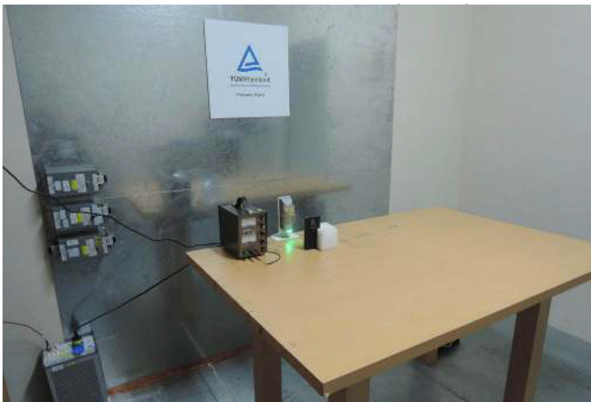
Photograph 5: Set-up for for Mains Conducted testing Front
