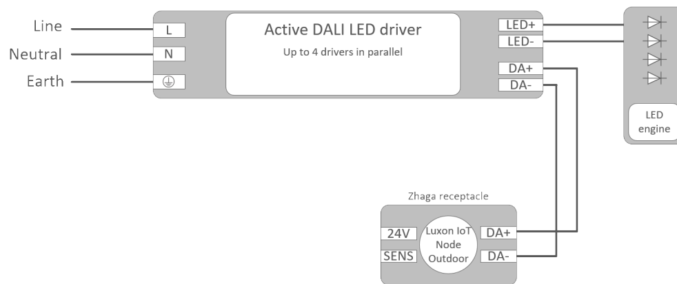
Wiring diagram 1: Active DALI application with Luxon IoT Node Outdoor
