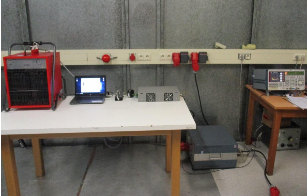
Photo 3: Photograph conducted emissions 0.15-30 MHz
