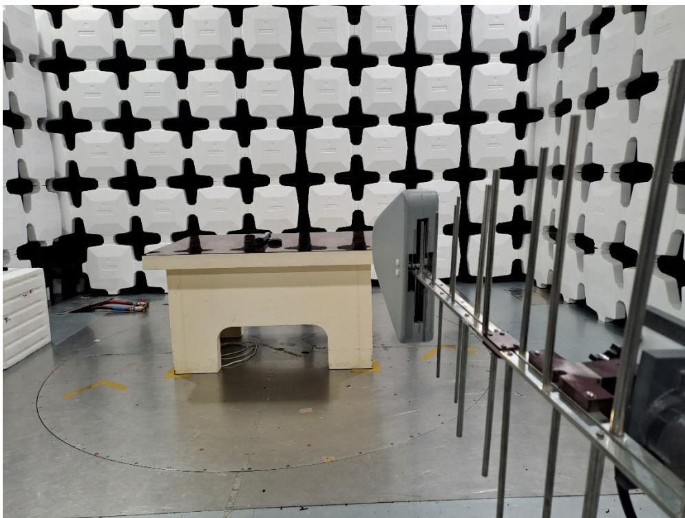
Photo 2 Photograph test setup radiated emissions 250-1000 MHz, report section 3.1
