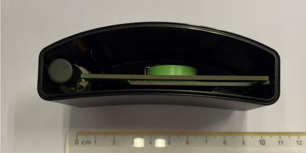
Fig. 4 - PCB and optional LF coil inserted in the housing of the sub assembly
