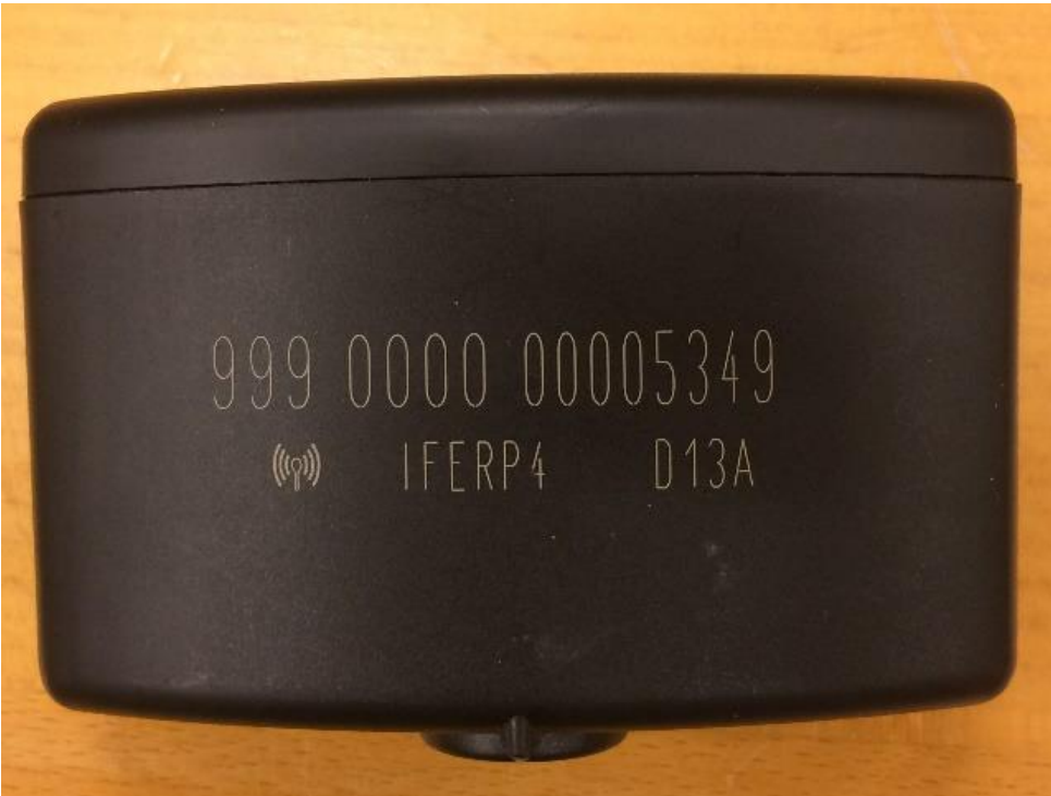
Fig. 5 – Subassembly after potting and ultrasonic welding
