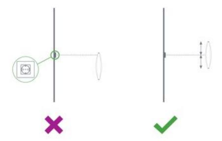
Before the installation, it is advised to gain information on the flooring that is below the antenna. If a dry-walk floor mat is used, it might have metal components that influence RF detection performance. In that case a cut needs to be made in the floor mat to break conduction between the metal components in the mat and the antenna.
