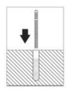
Always use a nylon insulation ring to insulate the gate from the floor.
