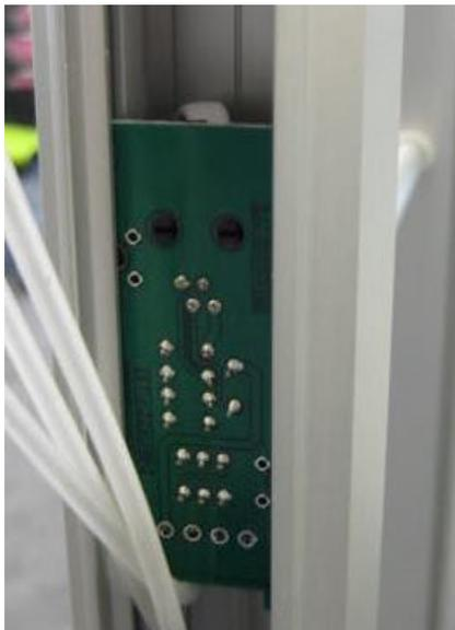
**Description of EUT:** Anti-Pilferage System operating in the band 7.400-8.800 MHz with antennas FL30 and FL45 including a metal detection module operating on 125 kHz with an option to communicate with the outside world via LAN
