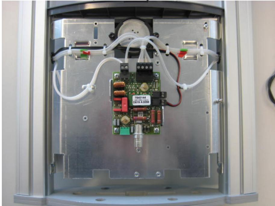
**Description of EUT:** Anti-Pilferage System operating in the band 7.400-8.800 MHz with antennas FL30 and FL45 including a metal detection module operating on 125 kHz with an option to communicate with the outside world via LAN
