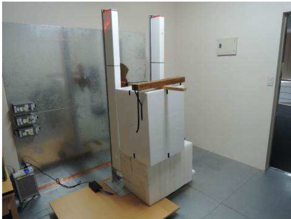
Photograph 5: Set-up for Mains Conducted testing Front
