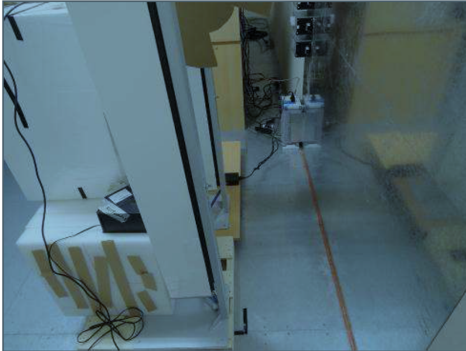
Photograph 4: Set-up for Mains Conducted testing Back
