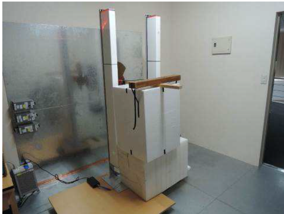
Photograph 5: Set-up for Mains Conducted testing Front
