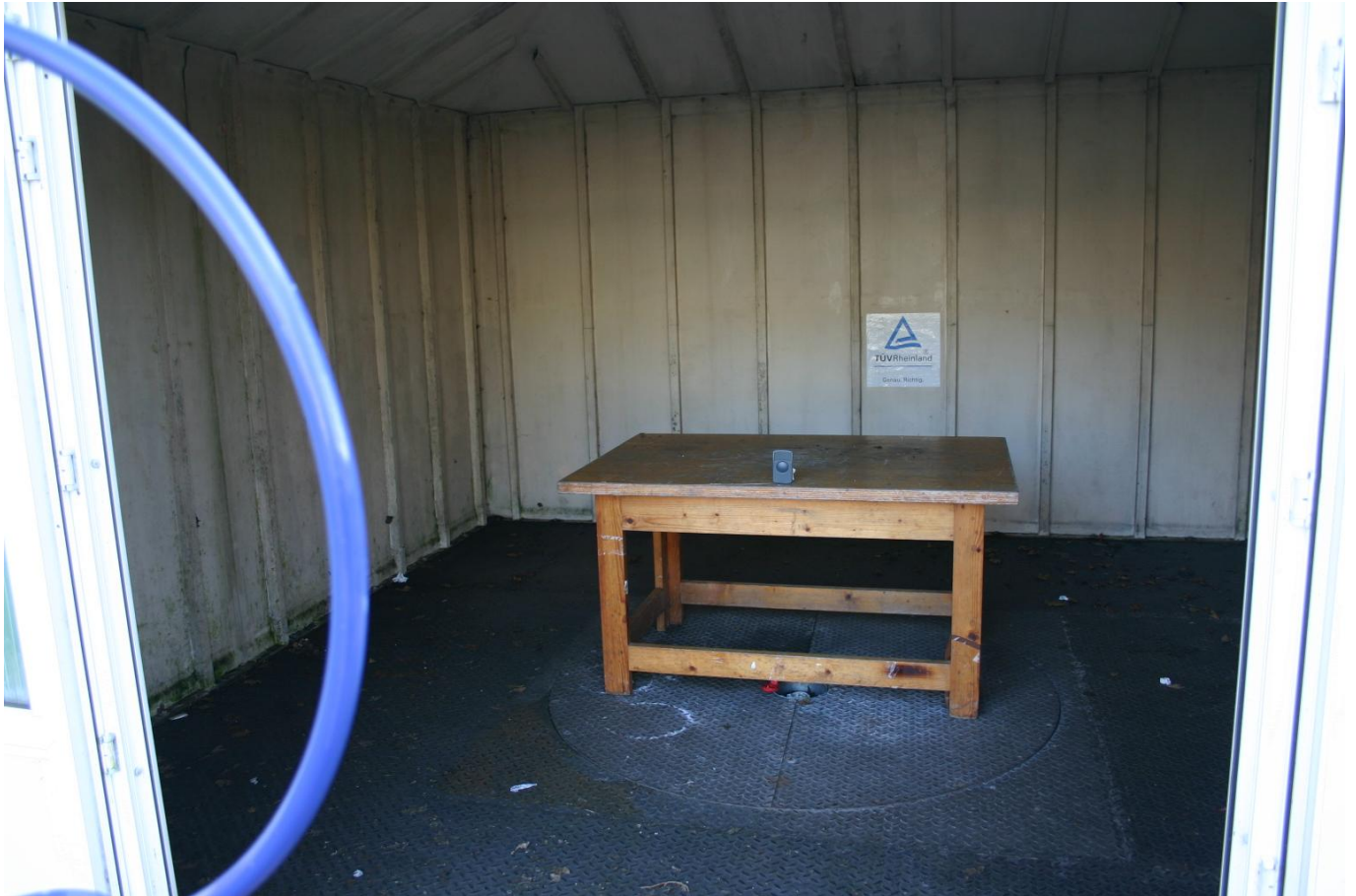
Radiated emission setup, Magnetic field
