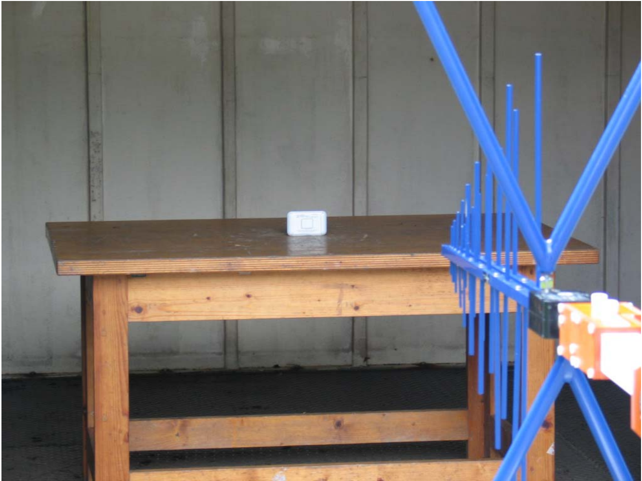
Photo 1: Radiated emission measurement set up
