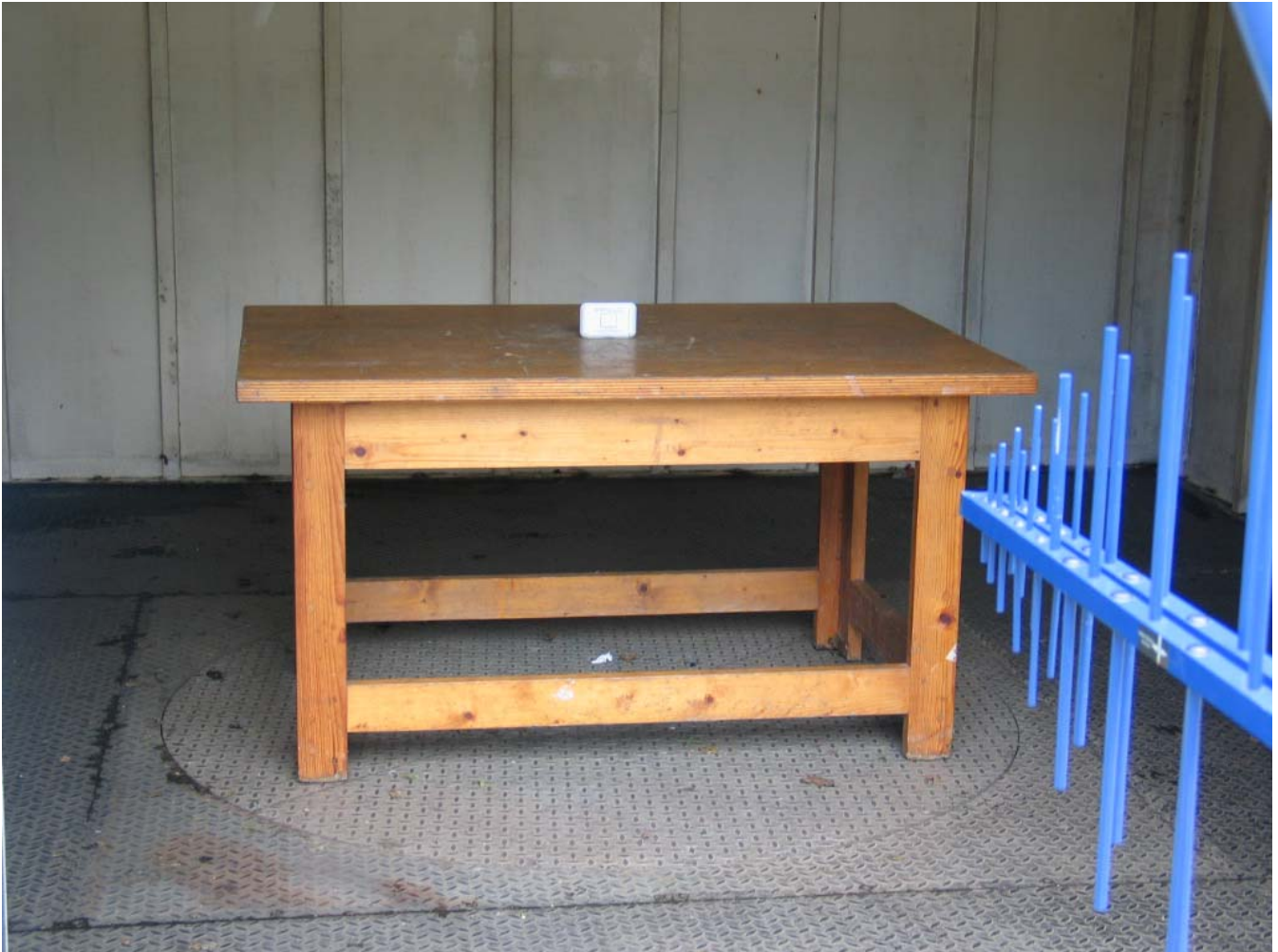
Photo 1: Radiated emission measurement set up
