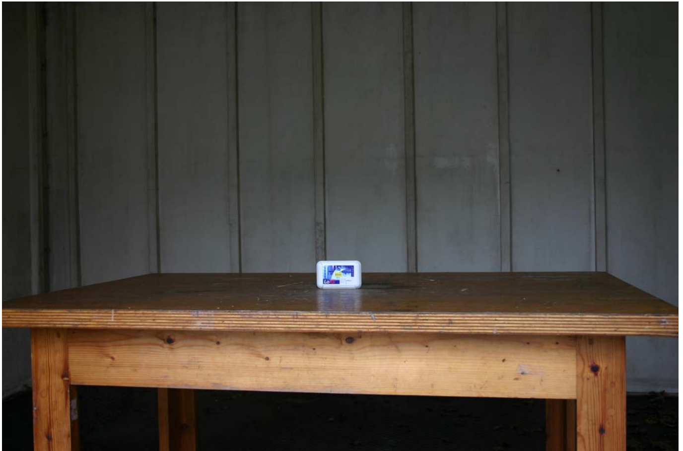
Photo 2: Radiated emission measurement set up; front side view
