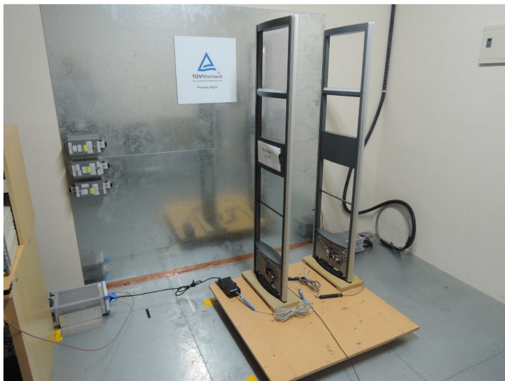
Photograph 5: Set-up for for Mains Conducted testing Front
